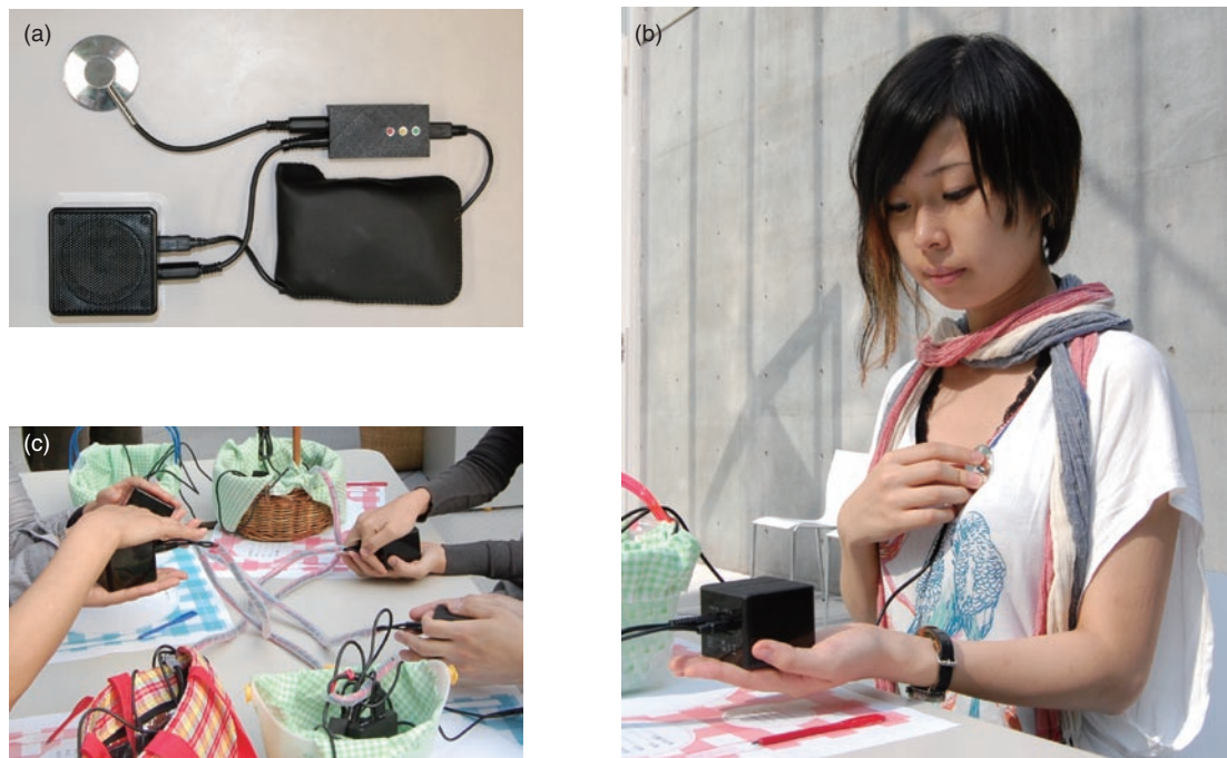
Fig. 4. (a) Equipment used in the workshop: stethoscope, vibration speaker (heart box), signal processing circuit, and batteries. (b) Equipment in use. (c) Exchange of heart boxes among participants.
