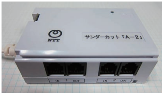
Photo 1. Lightning protection adaptor for analog port.
