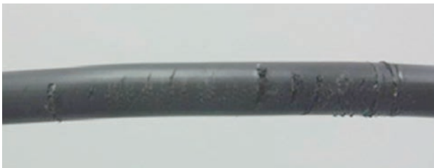
Fig. 4. Cable damaged by a sharp-edged object.
