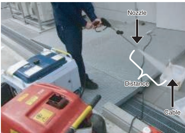
Fig. 5. Damage-reproduction experiment using a high-pressure water sprayer.
