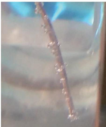
Fig. 6. Exposure to sunlight produces reaction gases (mainly hydrogen) on the electrode (rod).
