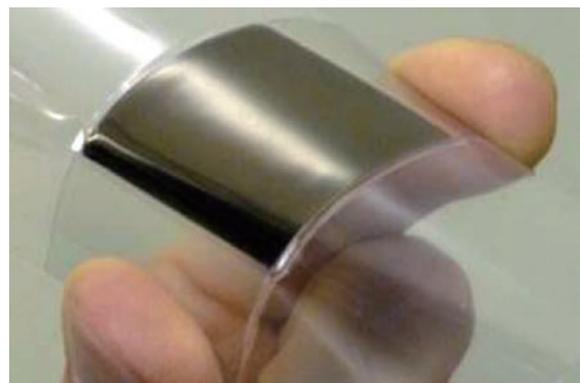
Fig. 10. Thermoelectric element (1 square inch).
