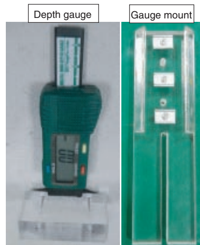
Fig. 5. SP near-ground wastage measurement tool.
