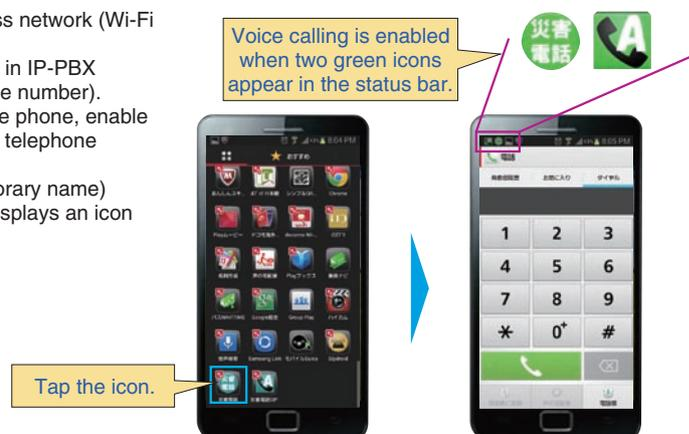
Fig. 1. IP phone application for smartphones.
