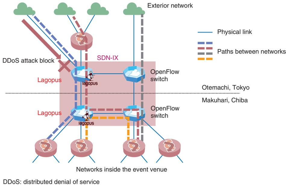
Fig. 2. Network configuration of SDN-IX for Interop Tokyo 2015 ShowNet.
