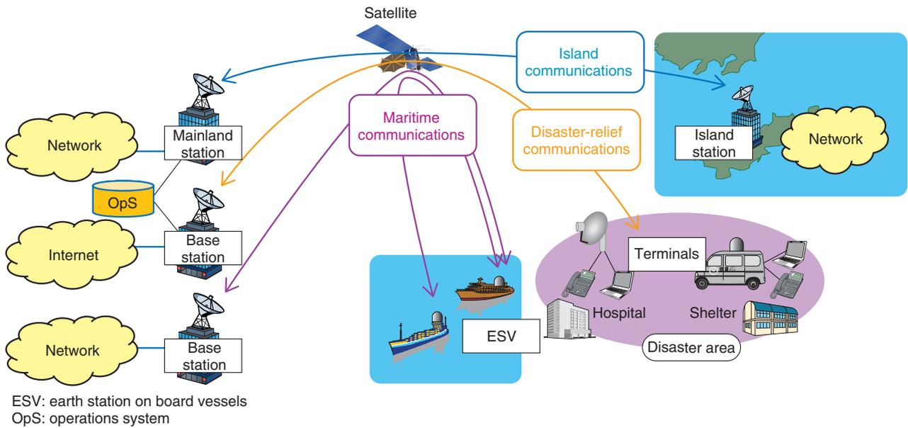
Fig. 1. Highly Efficient Satellite Communication System (HESCS).
