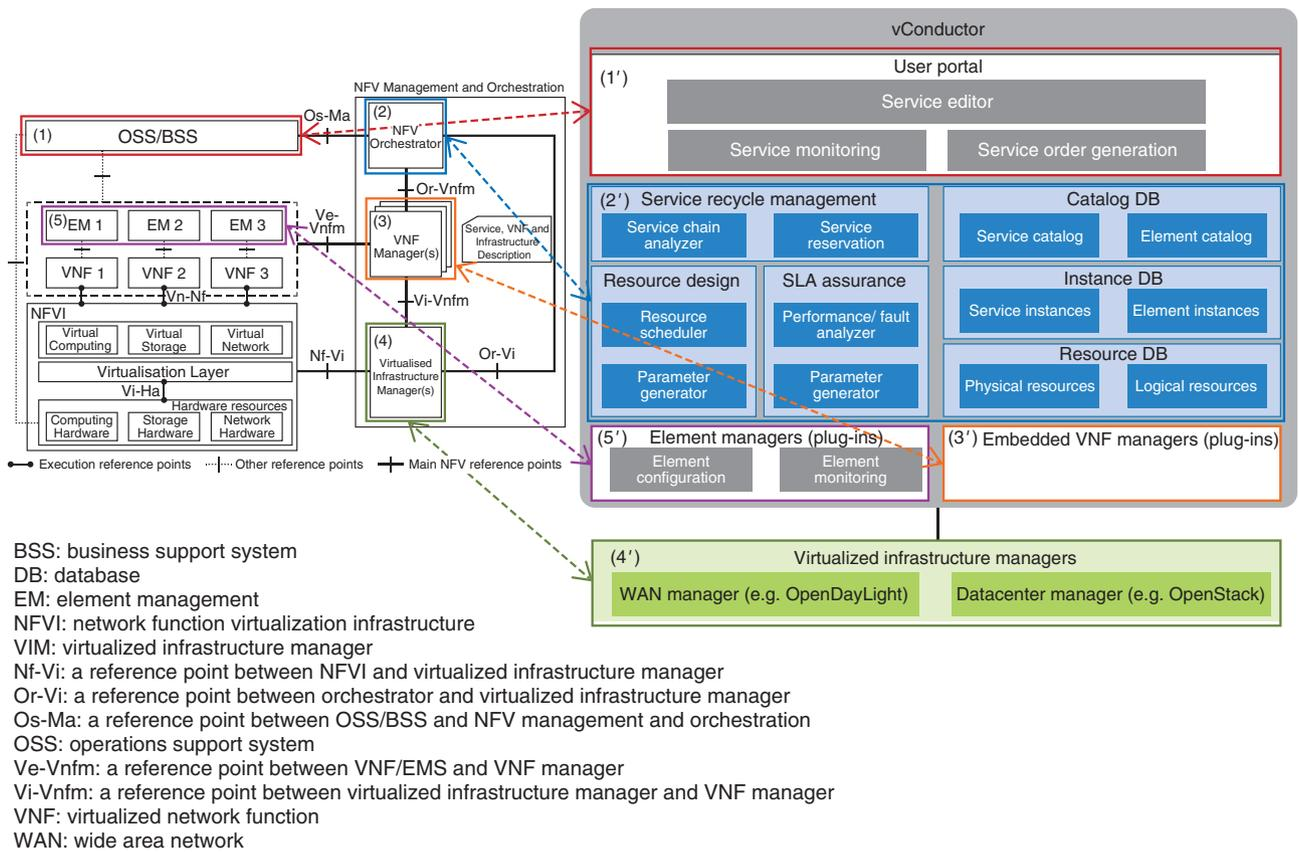
Fig. 5. Relationship between NFV reference architecture framework and vConductor system structure.
