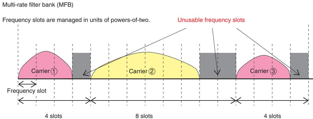
Fig. 3. Problem of unused frequency slots with GMM.
