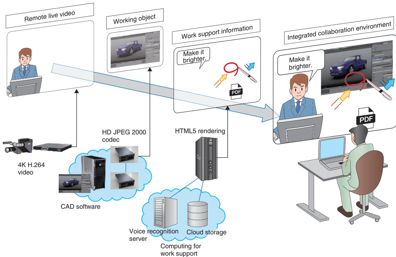
Fig. 4. Overview and application example of Augmentation Layer.
