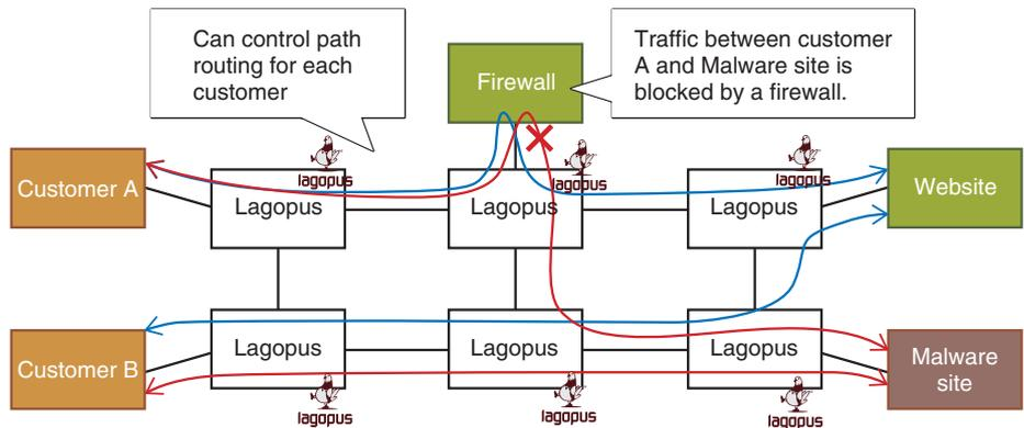
Fig. 3. Example of segment routing traffic control.
