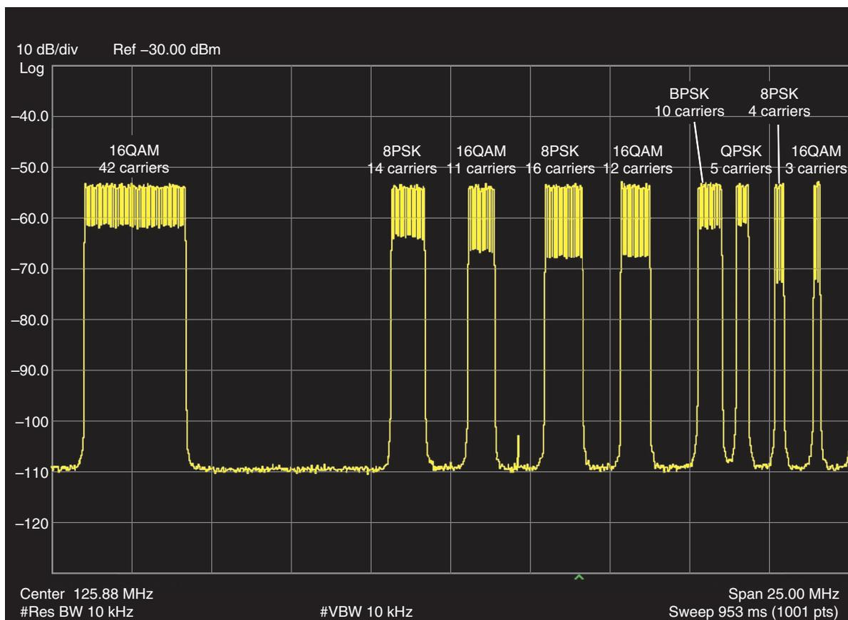
Fig. 7. Transmission of multi-channel multi-carrier signals.
