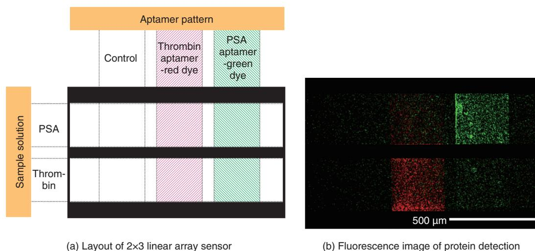
Fig. 3. Demonstration of simultaneous multiple protein detection.
