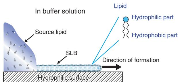
Fig. 1. Fabrication of SLB by self-spreading technique.
