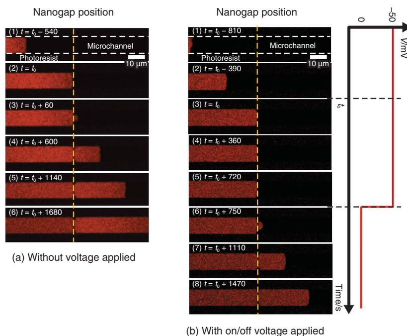
Red fluorescence is SLB. White dotted horizontal line indicates 10- $\mu\text{m}$ -wide line pattern, and yellow dotted vertical line indicates nanogap position. The time at which SLB reached the nanogap position is set as  $t_0$ .
