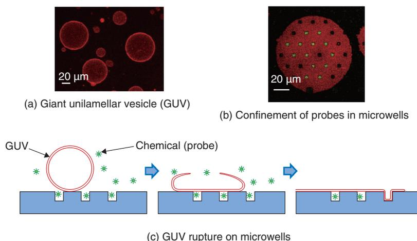
Fig. 2. Fabrication of microwells sealed with a lipid membrane.
