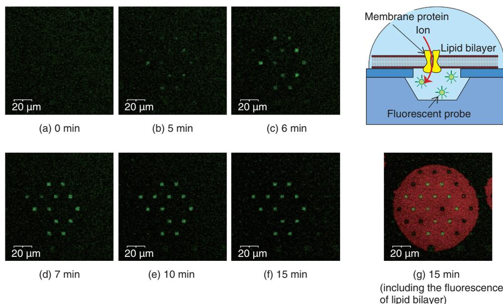
Fig. 3. Functional analysis of  $\alpha$ -hemolysin with fluorescent microscopy.
