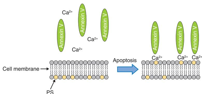
Fig. 4. Detection of PS translocation using Annexin V.
