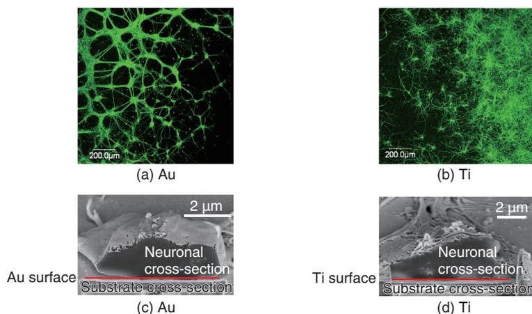
Fig. 2. Microscopic images of neurons cultivated on Au and Ti surfaces. Red lines show the substrate surface [2].
