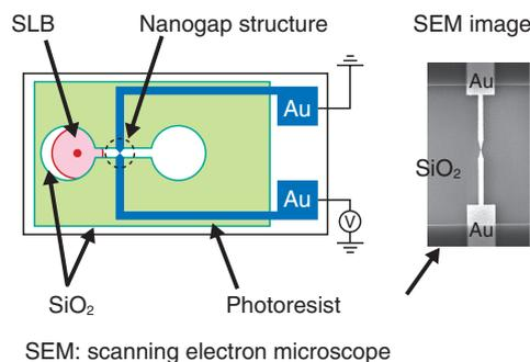
Fig. 4. Design of new pattern with nanogap structure.
