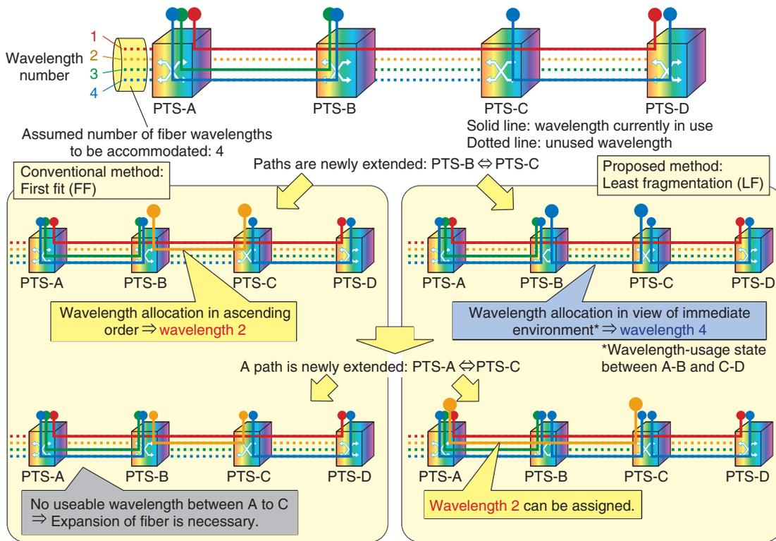
Fig. 4. Improved accommodation efficiency by LF algorithm.
