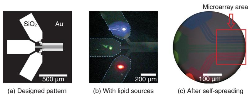
Fig. 2. Fabrication of dense SLB microarray.
