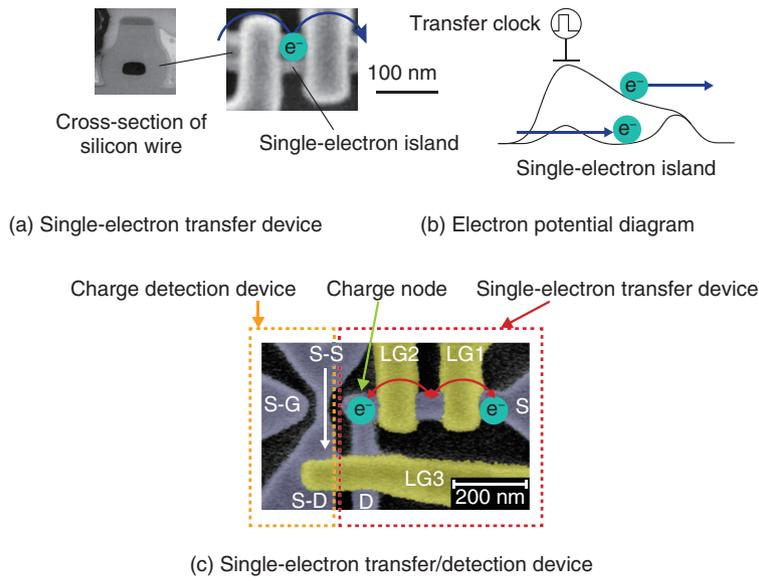
Fig. 2. Single-electron transfer and detection using silicon transistors.
