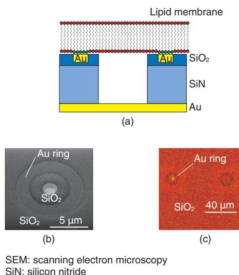
Fig. 5. (a) Schematic illustration of microwell structure. (b) SEM image of the Au ring substrate. (c) Fluorescence from the rhodamine-B labeled lipid membrane. The green fluorescent probe is confined in the microwell.
