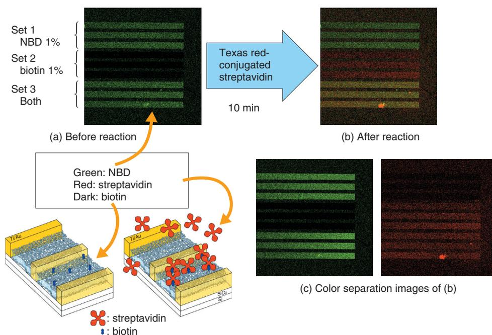
Fig. 3. Demonstration of protein detection with SLB microarray.
