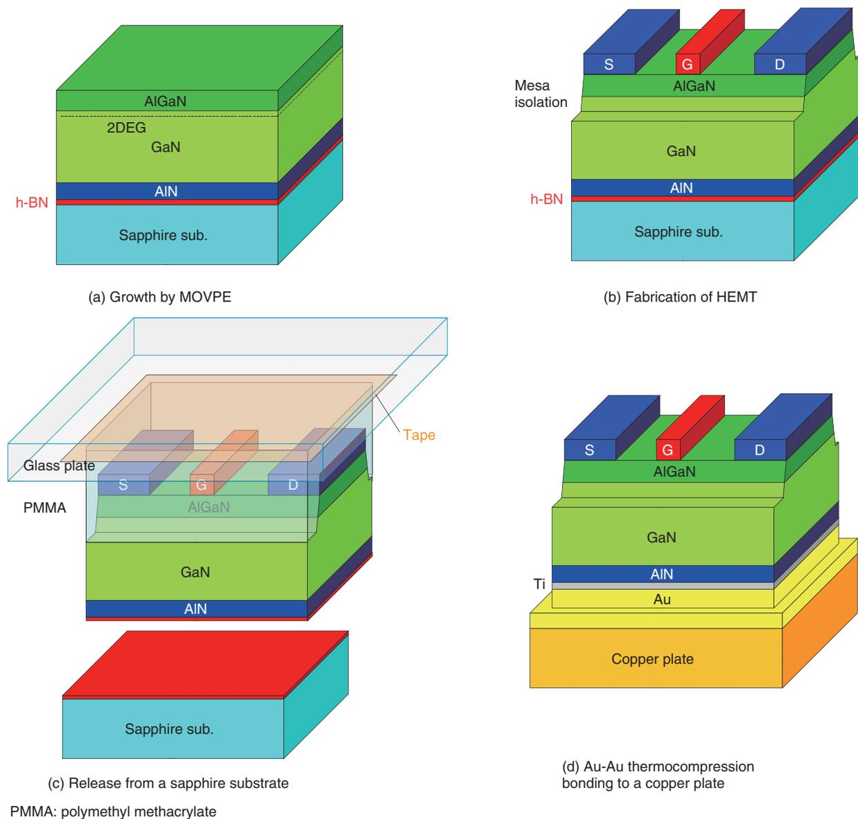
Fig. 2. Schematic views of h-BN ELO and transfer processes of AlGaN/GaN HEMT. (a) Growth of AlGaN/GaN heterostructures on AlN NL deposited on h-N/sapphire. (b) Fabrication of AlGaN/GaN HEMTs by conventional photolithography and lift-off technique. The labels S, G, and D indicate source, gate, and drain electrodes, respectively. (c) Mechanical ELO of the HEMTs from sapphire substrate. (d) Transfer of the HEMTs to a copper plate by Au-Au thermocompression bonding.
