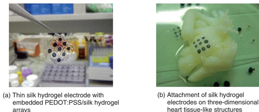
Fig. 4. Large-scale PEDOT:PSS/silk composite electrodes.
