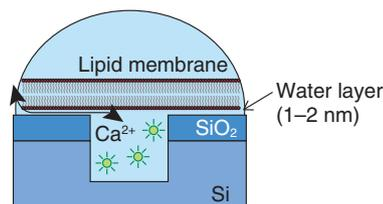
Fig. 4. Schematic illustration of microwell structure sealed by a lipid bilayer showing the passage of  $\text{Ca}^{2+}$  through the water layer.
