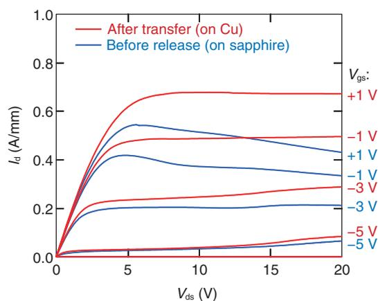
Fig. 4.  $I_d$ - $V_{ds}$  characteristics of AlGaIn/GaN HEMT before release and after transfer.
