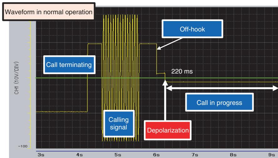
Fig. 5. Voltage between L1-L2 lines in normal connection.
