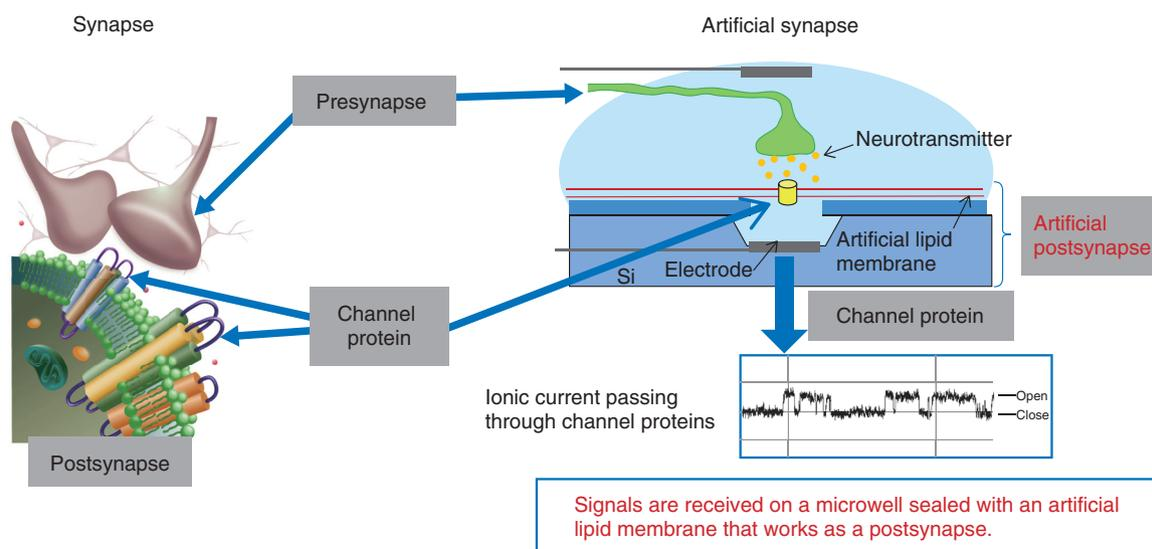
Fig. 1. Nanobiodevice that mimics the neuronal transmission mechanism.
