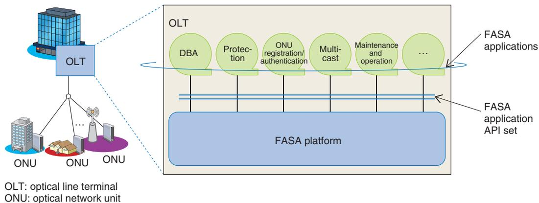
Fig. 1. Concept and component of modularization by FASA.
