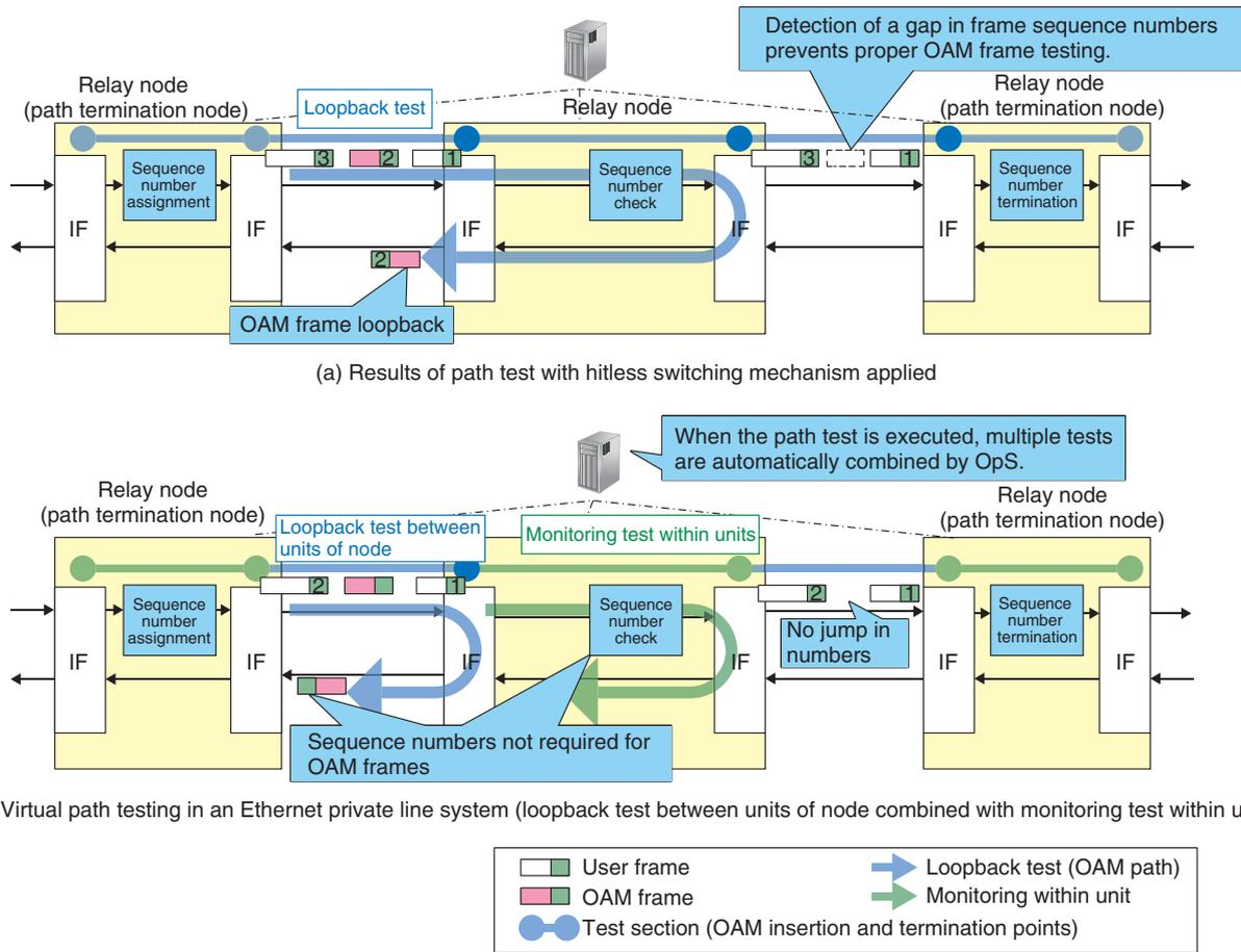
Fig. 4. Virtual path testing.
