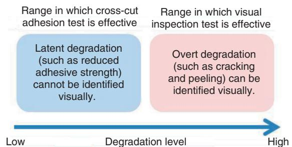
Fig. 5. Effective ranges in which cross-cut adhesion test and visual inspection are effective.
