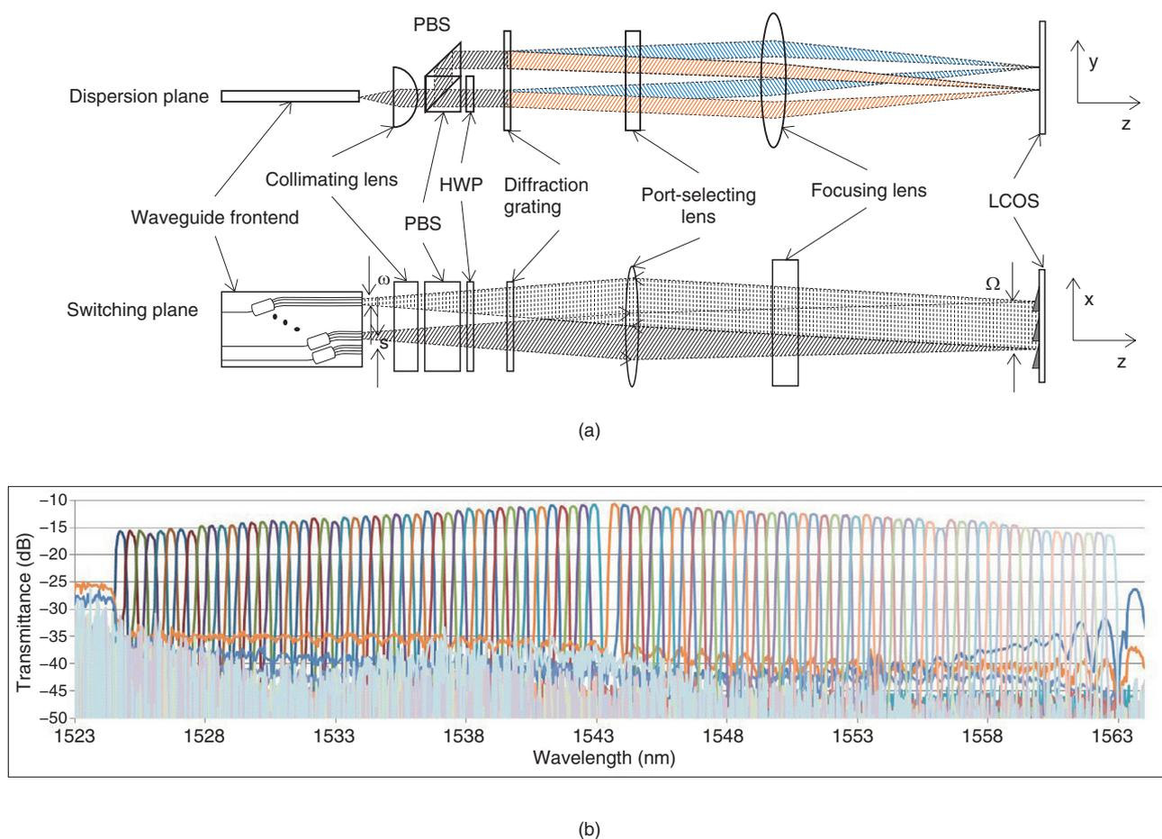
Fig. 5. (a) Optical system schematics of a  $1 \times 95$  WSS in two orthogonal projections. (b) Superimposed transmission spectra of 95 curves that were taken at the different ports.
