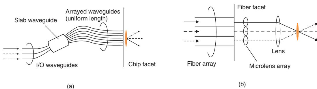
Fig. 2. Optical frontend configurations: (a) SBT circuit for launching three beams with different angles from the same position at the chip facet. (b) Equivalent optical design based on conventional discrete lenses.
