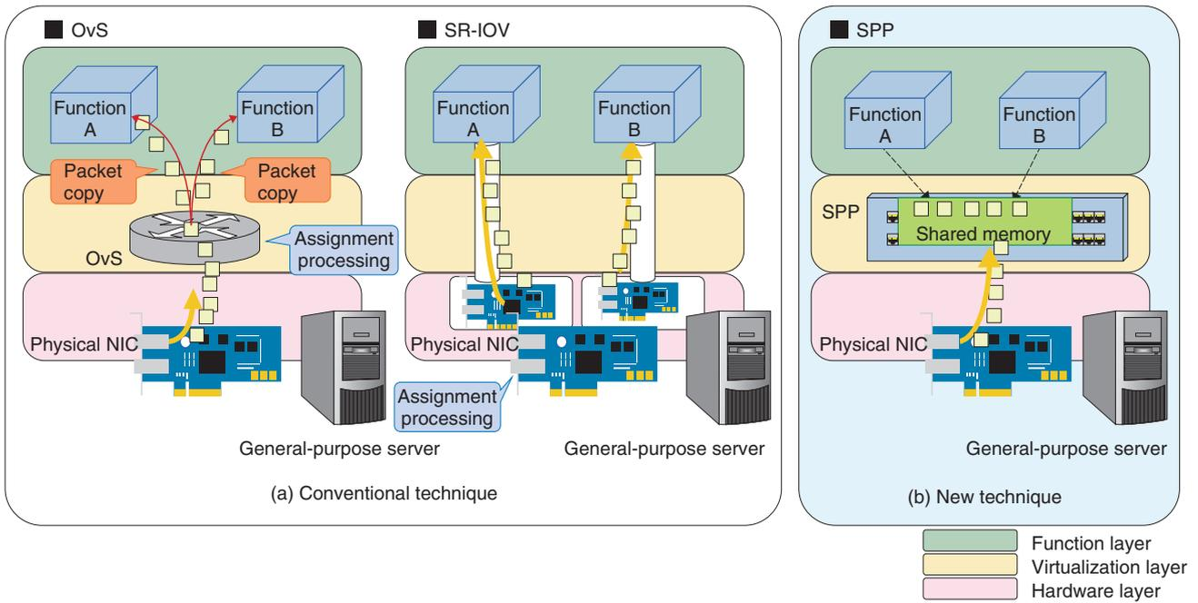
Fig. 2. Configuration image of SPP and conventional technique.
