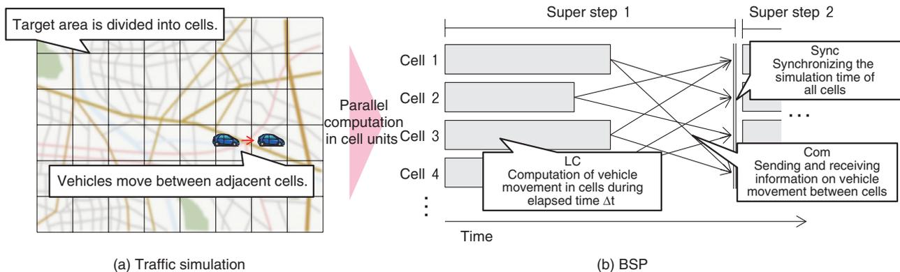
Fig. 2. Model for processing traffic simulation.
