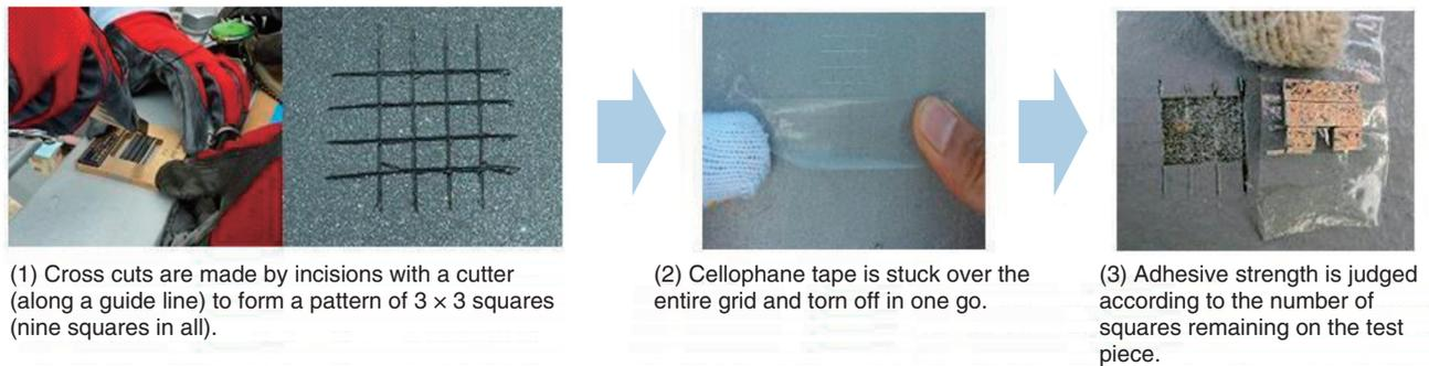
Fig. 4. Procedure of cross-cut adhesion test.
