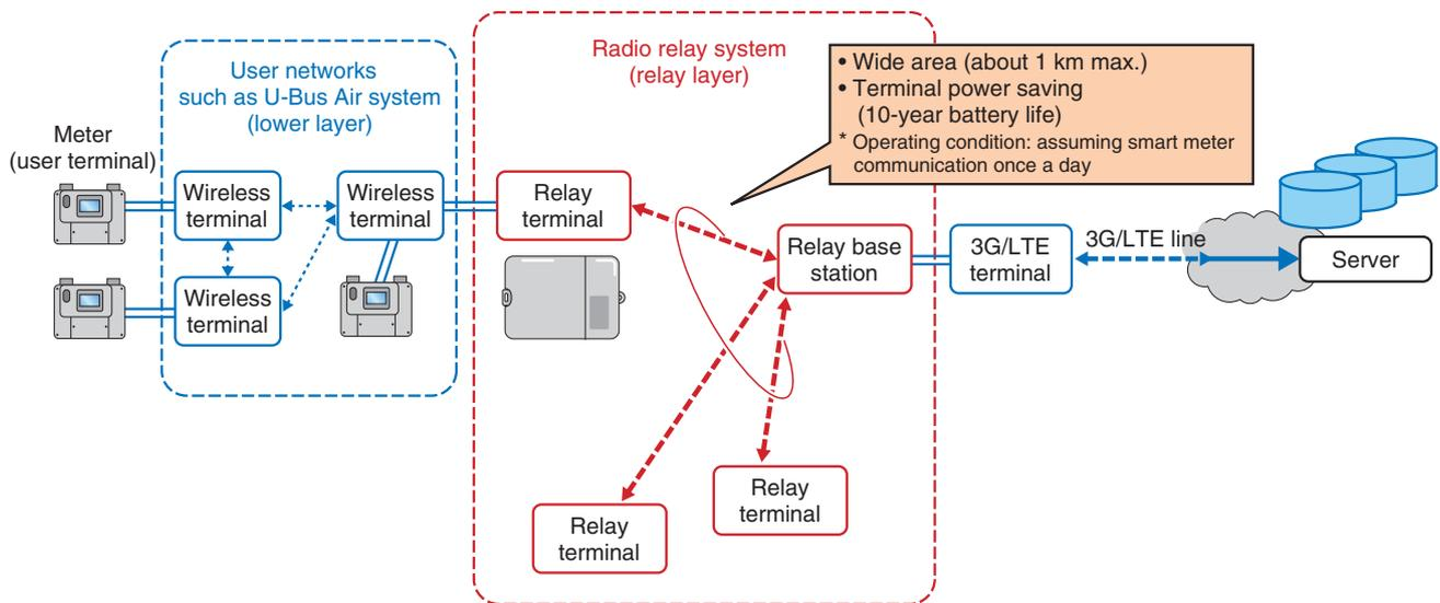
Fig. 3. System configuration of radio relay system.
