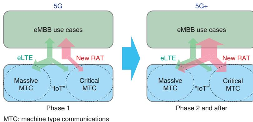
Fig. 3. 5G phased approach from use case perspective.
