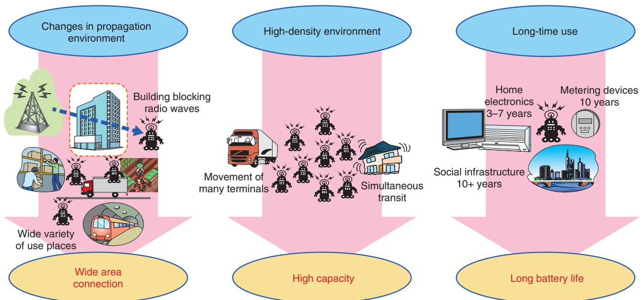
Fig. 1. Typical communication environment expected for IoT/M2M services.
