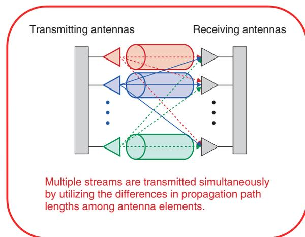
Fig. 2. System image: using short range MIMO techniques.
