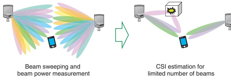
Fig. 6. Possible beamforming strategy for massive MIMO.
