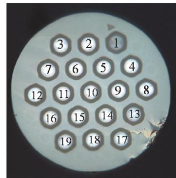
Cross section of fabricated optical fiber
