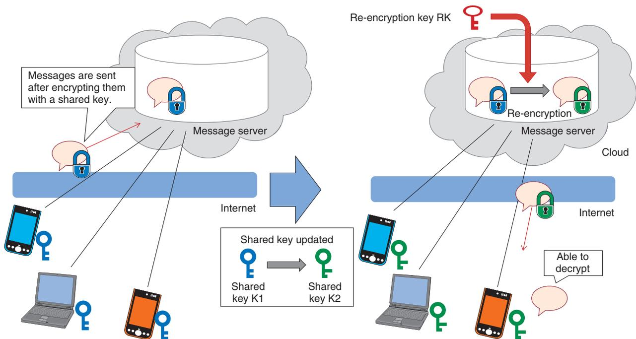
Fig. 3. Proxy re-encryption.
