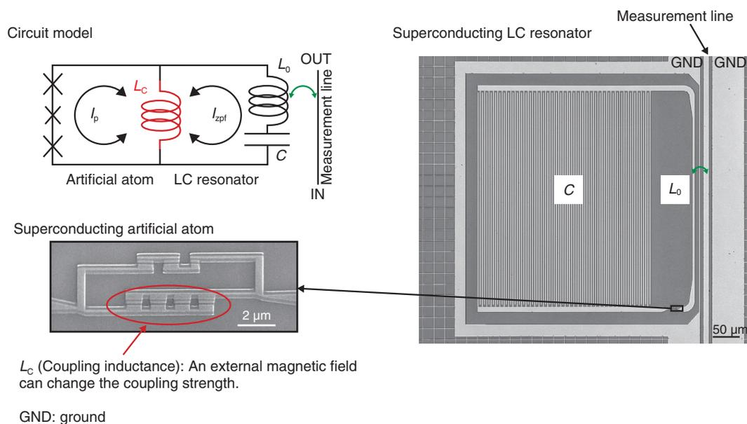
Fig. 3. Superconducting artificial atom – LC resonator coupled system.
