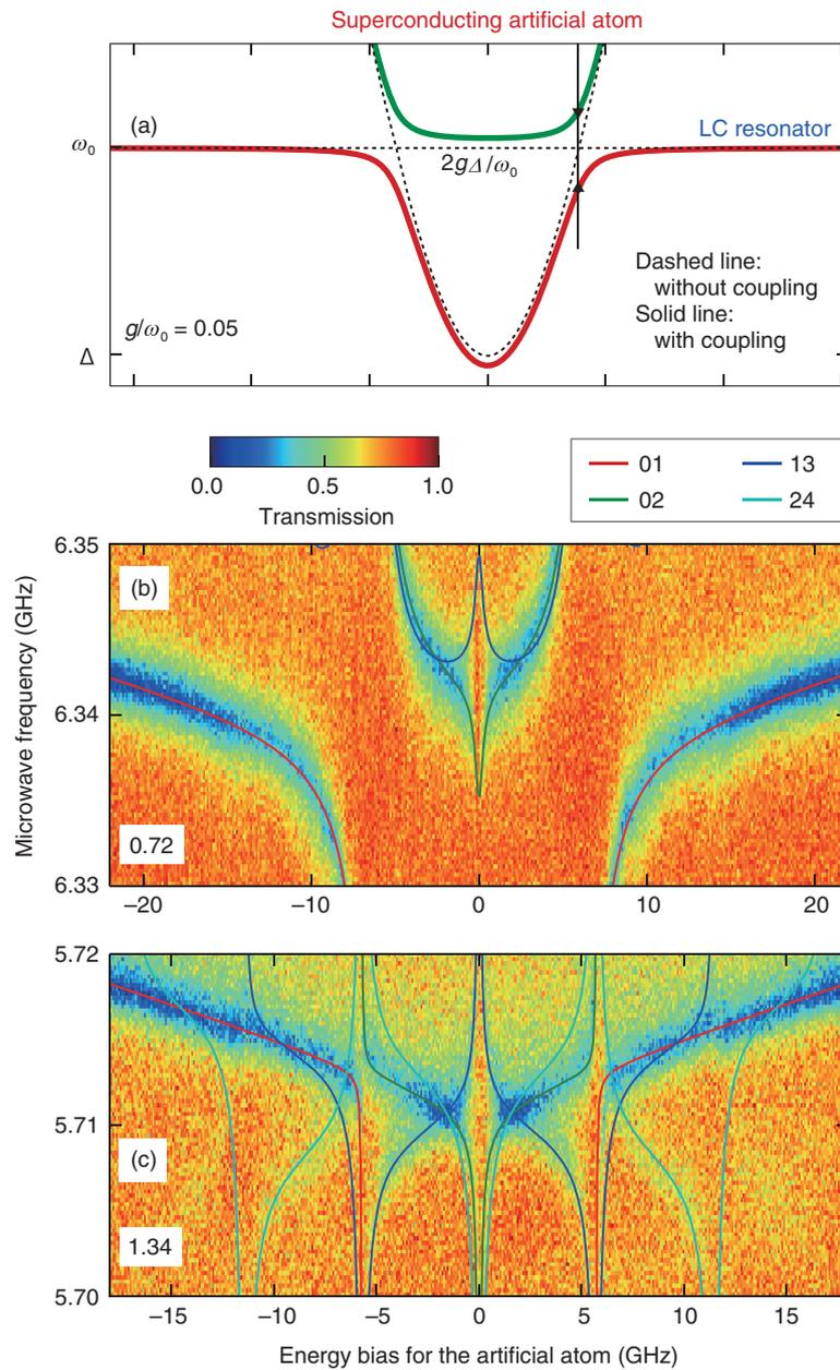
Fig. 4. Transmission spectra for the coupled system.
