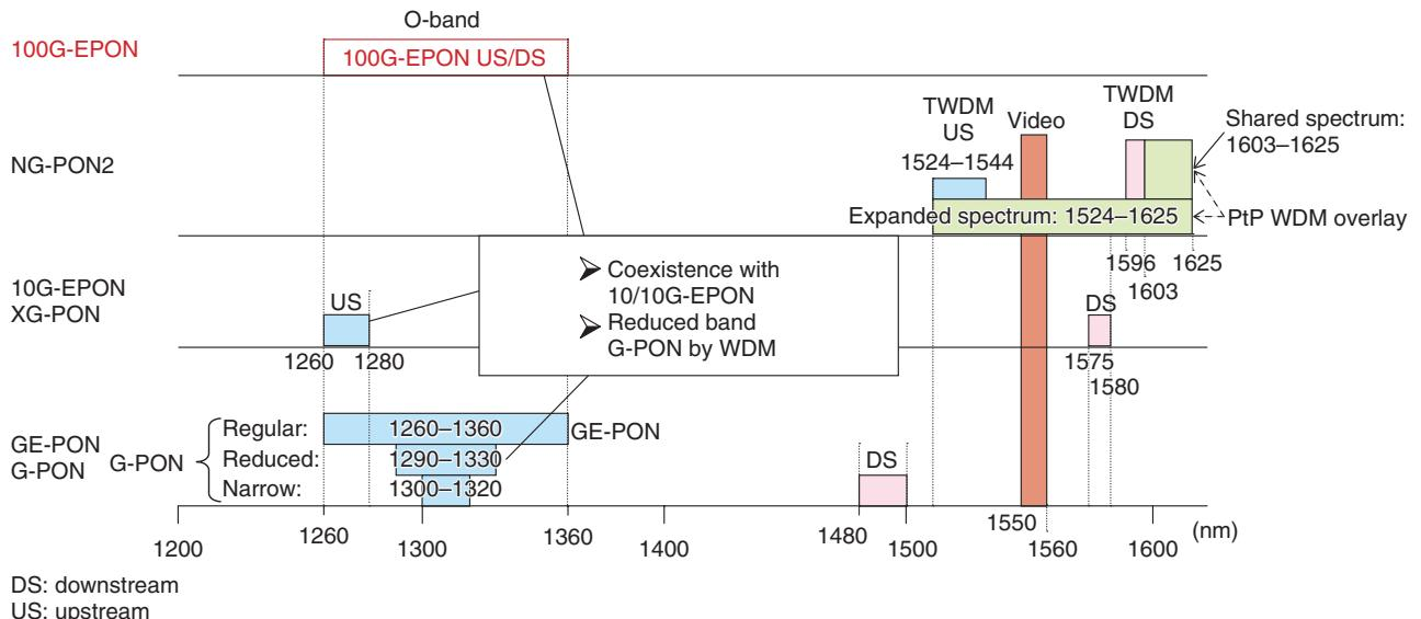
Fig. 3. A wavelength plan for 100G-EPON.
