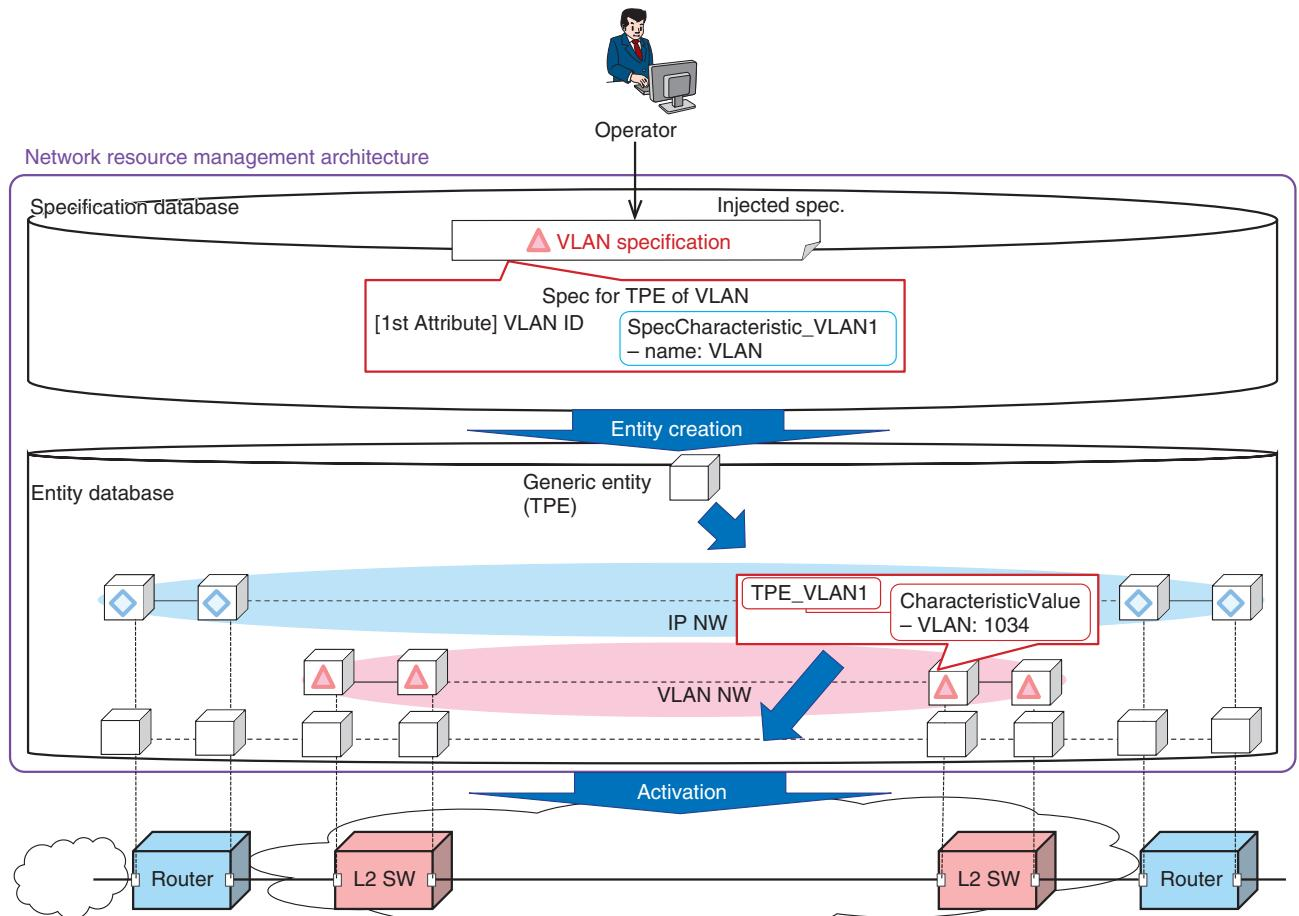
Fig. 6. Example of VLAN network.
