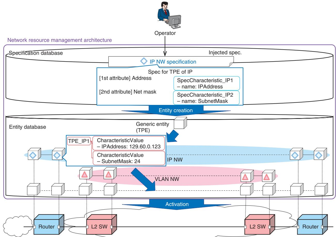
Fig. 5. Example of IP network.
