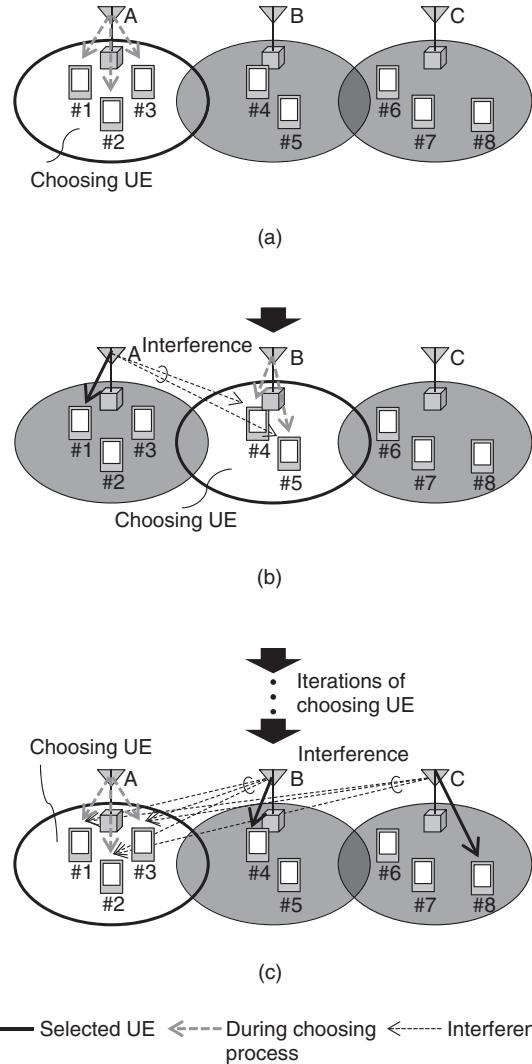
Fig. 2. Procedure for deciding the combination in the search process.
