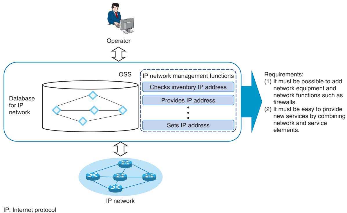
Fig. 1. Telecom operation and requirement for OSS.
