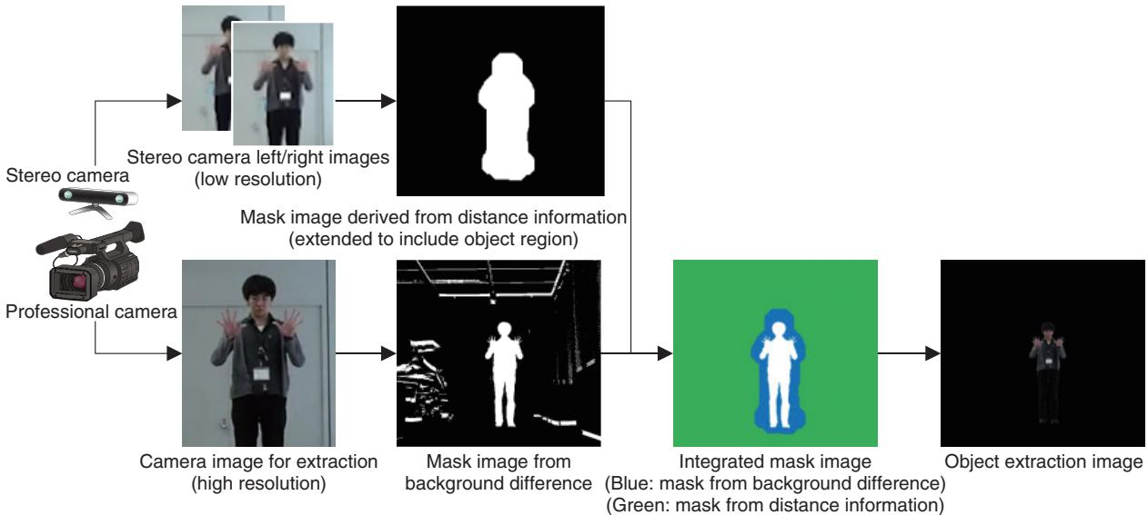
Fig. 3. Object extraction system incorporating a stereo camera.
