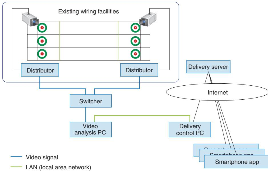
Fig. 4. Configuration of curling-stone location delivery system.
