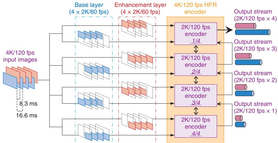
Fig. 3. System configuration.
