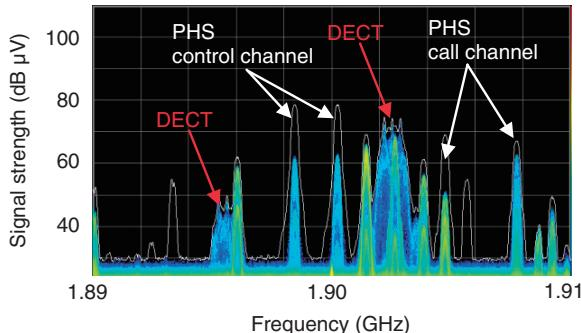
Fig. 4. Radio signal environment (measurement point A).
