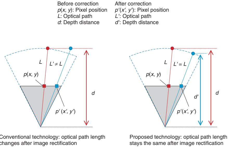
Fig. 3. Conceptual diagram of depth-image correction technology.
