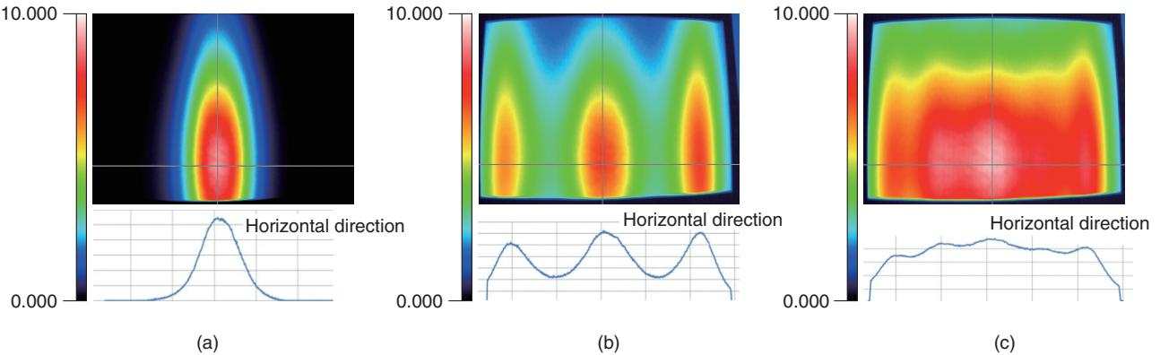
Fig. 5. Luminance distribution of obtained spatially imaged iris plane.
