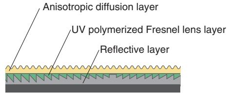
Fig. 4. Structure of spatially imaged iris plane screen.
