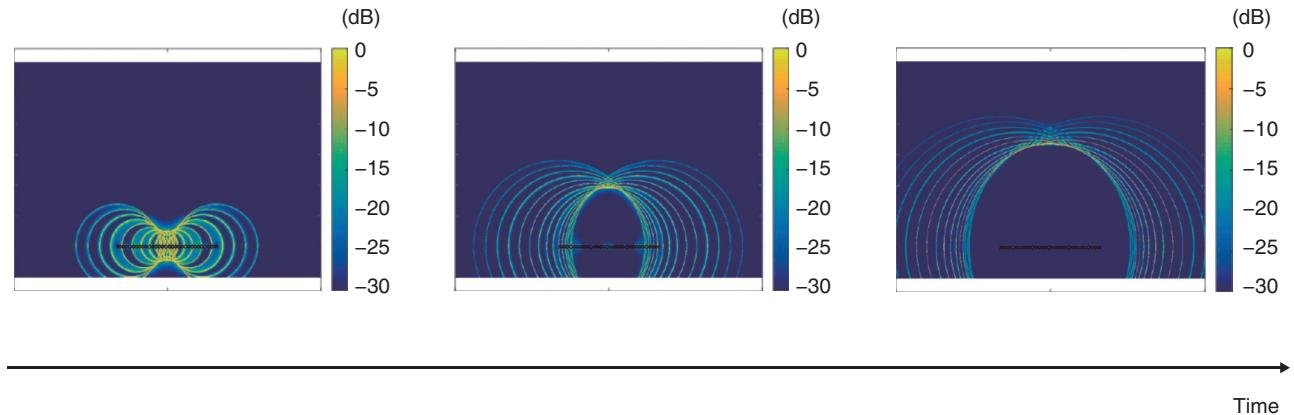
Fig. 4. Reproduced wave front using wave field synthesis.
