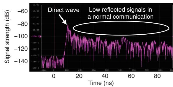
Fig. 8. Results of measuring reflected signals (normal communication).
