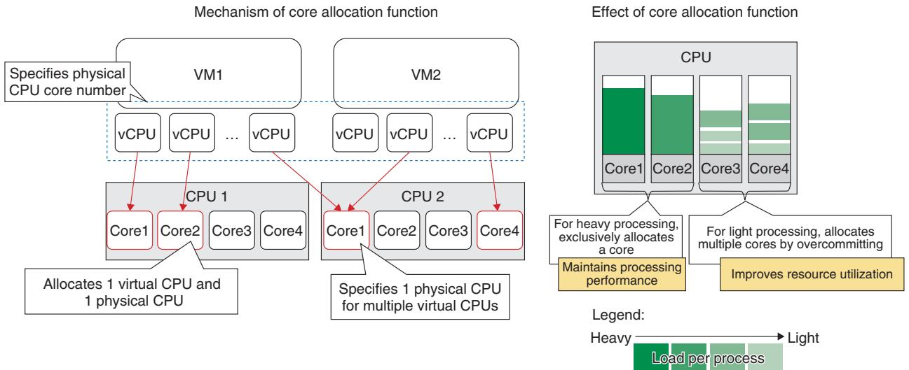
Fig. 3. CPU-core allocation function.
