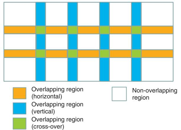
Fig. 2. Example of the overlapping regions used in 5(H) × 3(V) 4K video stitching.
