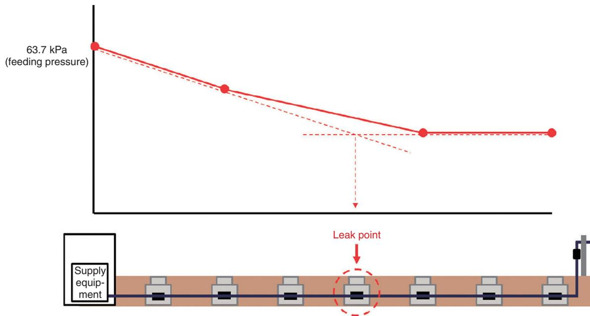
Fig. 5. Inference of gas leak point.
