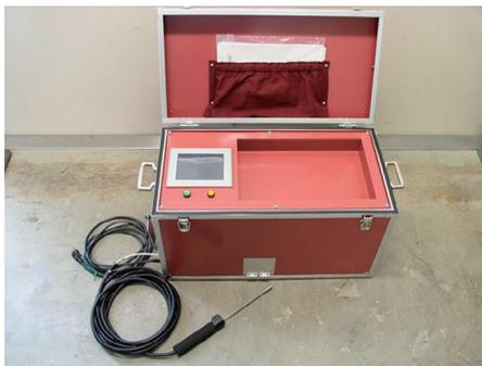
Fig. 8. Helium gas detection equipment.
