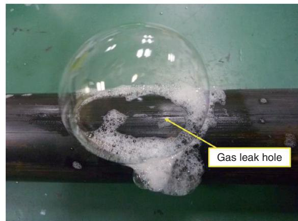
Fig. 6. Search for gas leak using soapy water.
