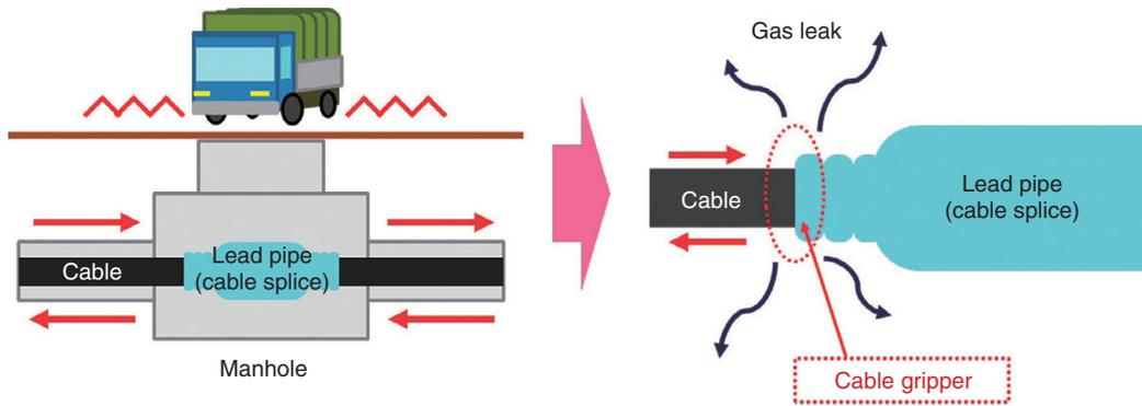
Fig. 2. Gas leak caused by cable movement.
