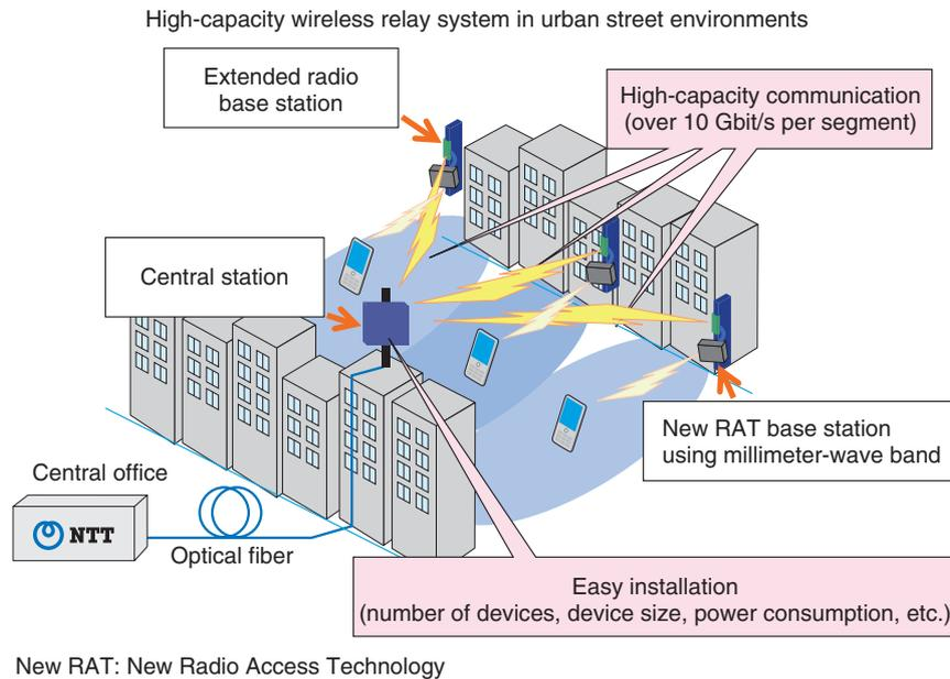
Fig. 2. High-capacity wireless relay technology.
