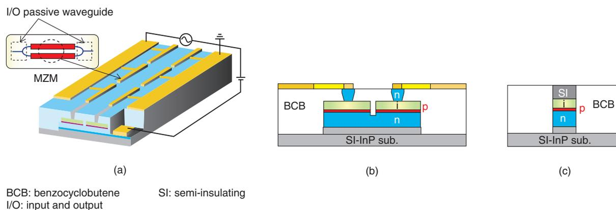
Fig. 1. Schematic illustration of (a) MZM, and cross-section diagrams of (b) its modulation region and (c) its I/O passive waveguide region.
