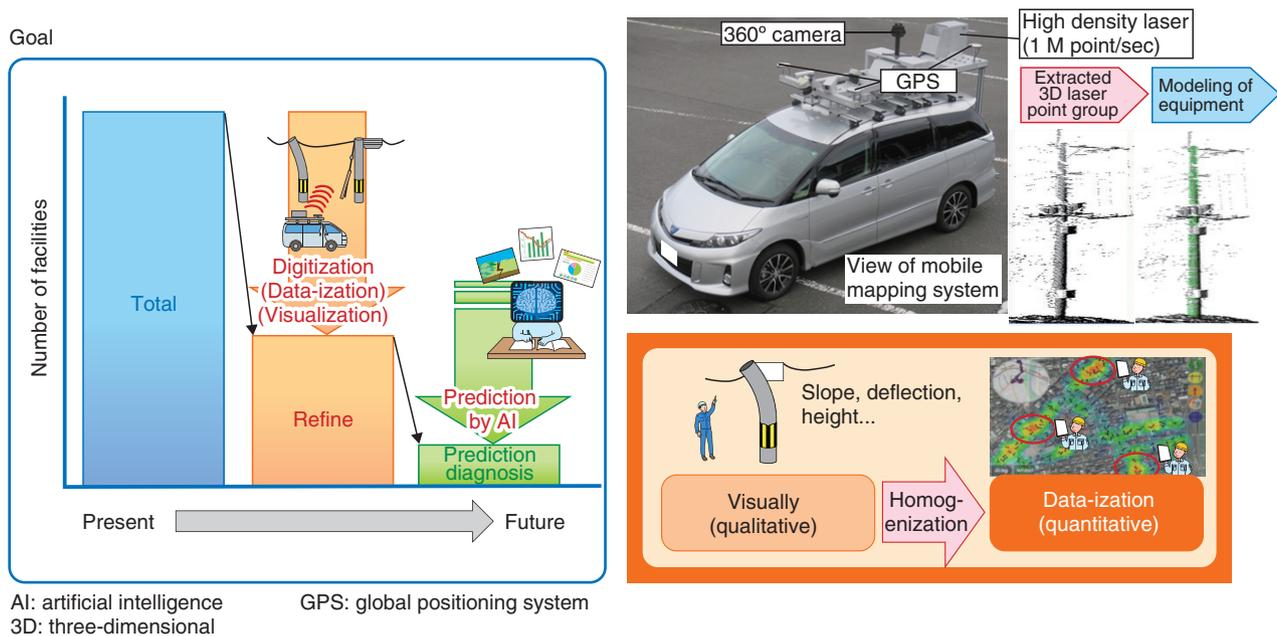
Fig. 1. Inspection technique for outdoor facilities.
