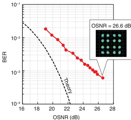
Fig. 10. Constellation diagram and BER characteristics of 64-Gbaud/16QAM.
