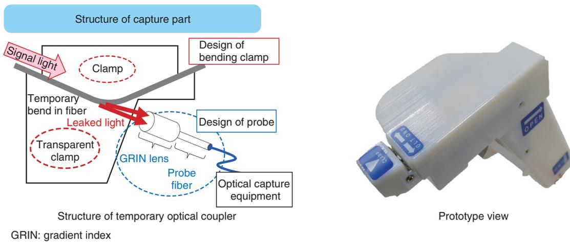
Fig. 3. Capturing MAC address of ONU signal using non-destructive fiber bending technique.
