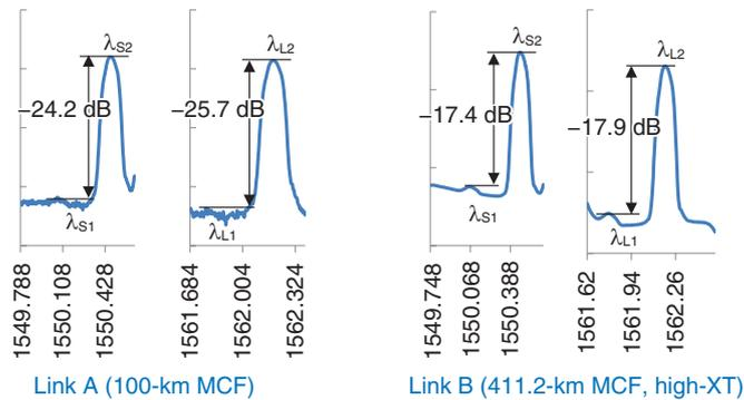
(b) Excerpt of pilot tone channels in Link A (c) Excerpt of pilot tone channels in Link B
