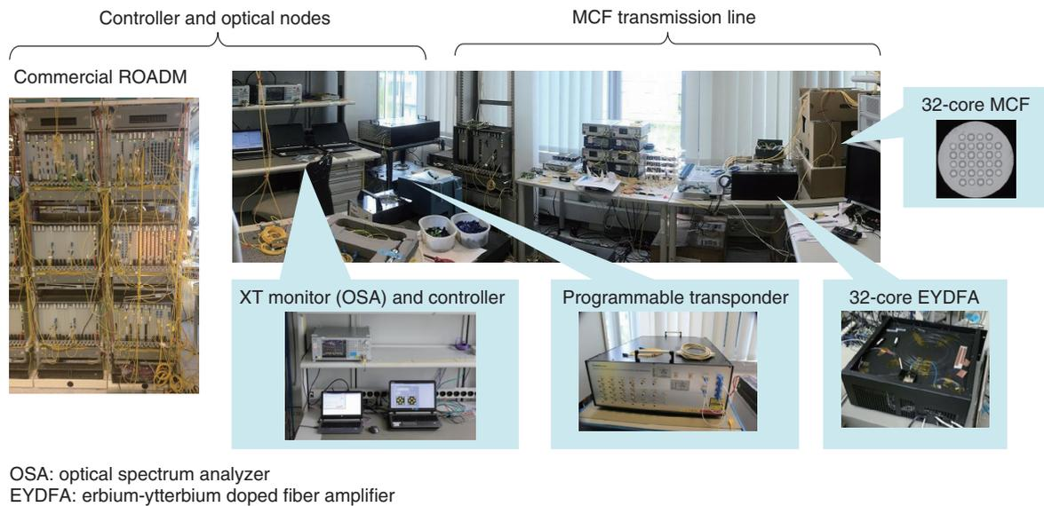
Fig. 3. Constructed testbed.
