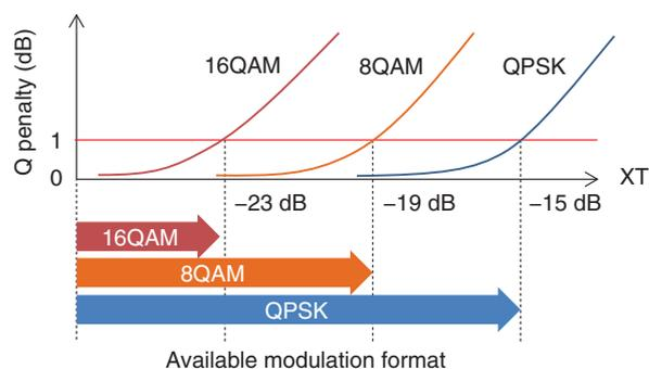
Fig. 2. Available modulation formats with respect to XT.
