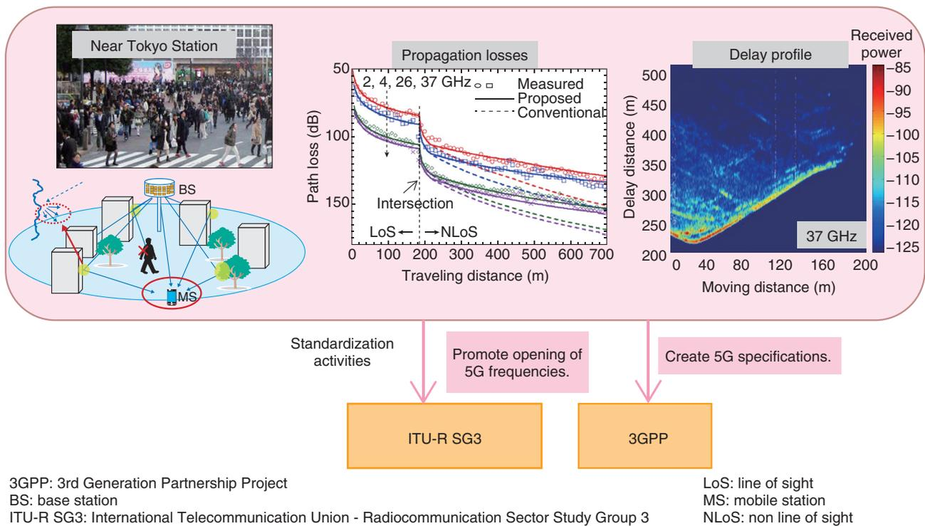
Fig. 4. Investigation of radio propagation models for 5G+.
