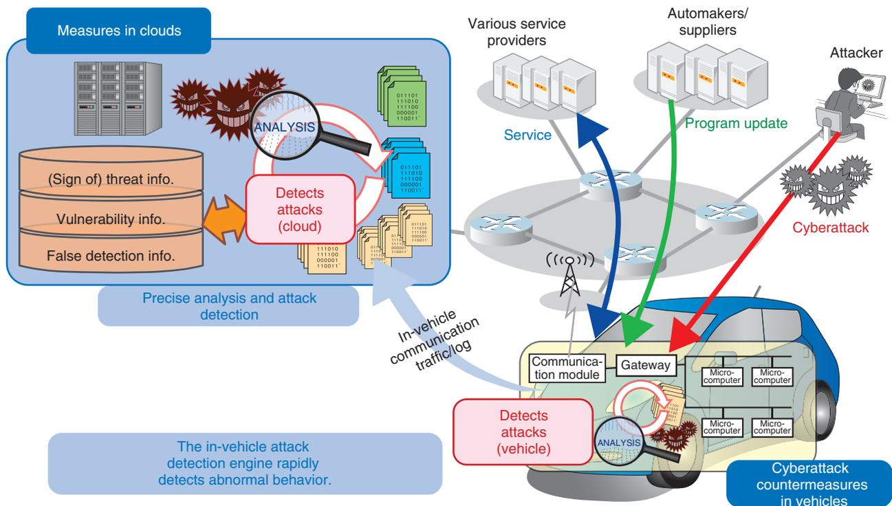
Fig. 10. Detection of cyberattacks on connected cars.
