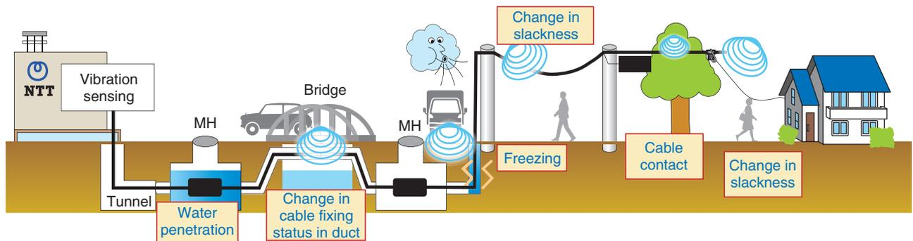
◆ Measured example of vibration sensing along cabled fiber
