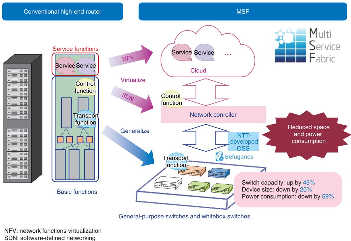
Fig. 12. Virtualization and generalization of high-end routers.
