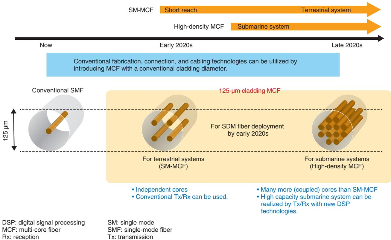
Fig. 5. SDM technology (multi-core and few-mode fibers).
