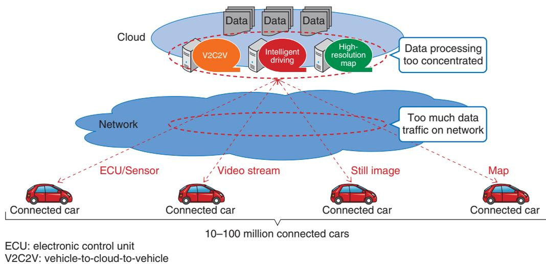
Fig. 1. Issues of current mobile network architecture [1].
