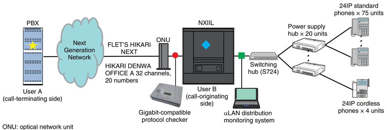
Fig. 1. Connection configuration and data collection points.
