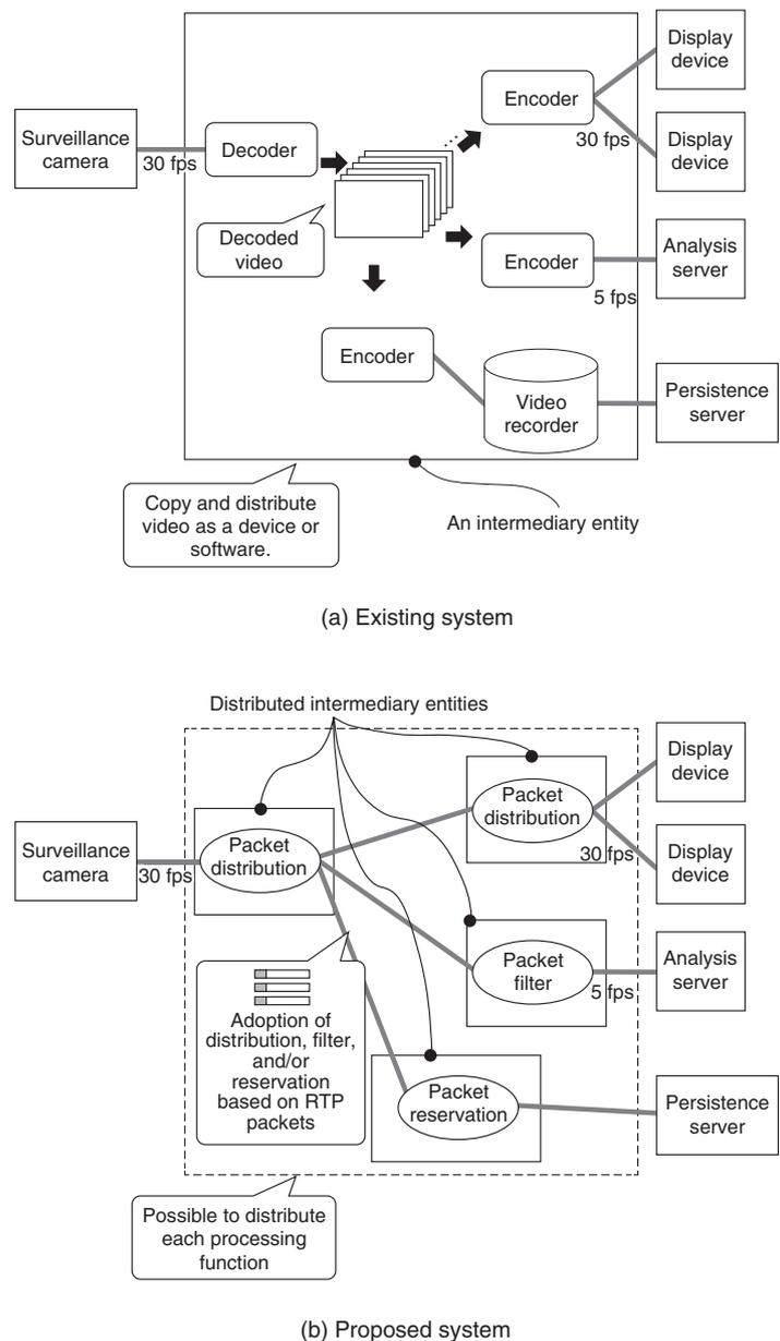
Fig. 3. Comparison of existing and proposed system architectures.
