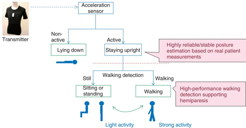
Fig. 6. Activity state estimation using acceleration data.
