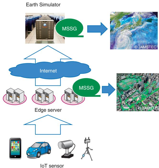
MSSG: Multi-Scale Simulator for the Geoenvironment (MSSG) weather forecasting software.
