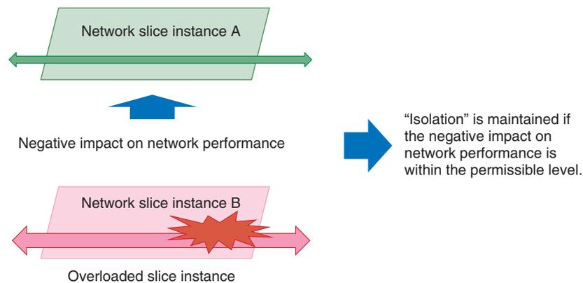
Fig. 2. Concept of isolation of network slice instances.
