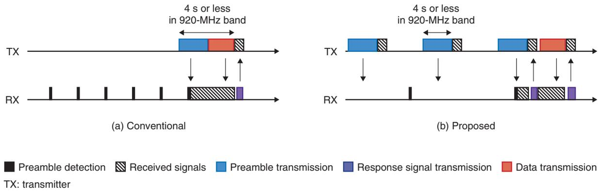
Fig. 4. Power saving standby operations.
