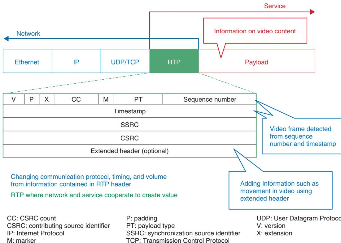
Fig. 2. Application example of network and service cooperatively using RTP.
