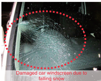
Fig. 3. Property damage accident caused by snow falling from overhead equipment.
