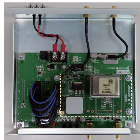
Inside the prototype GNSS receiver (Dashed line indicating the FURUNO GF-8705 GNSS receiver module)
