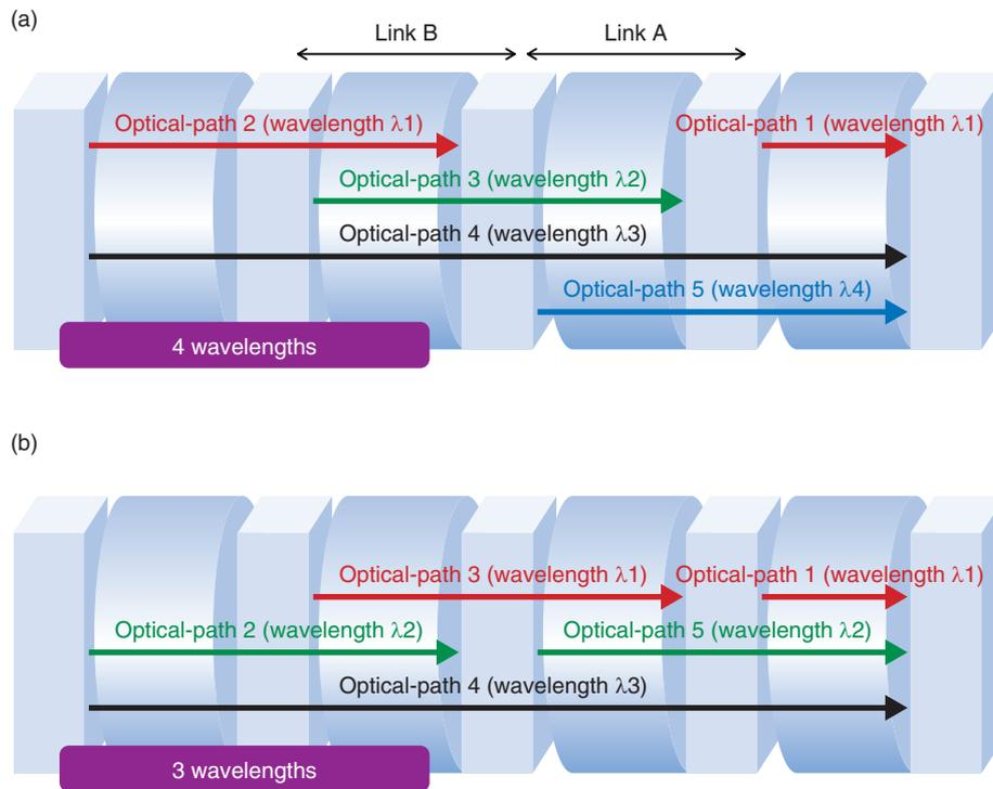
Fig. 1. Allocation of wavelengths to optical paths.
