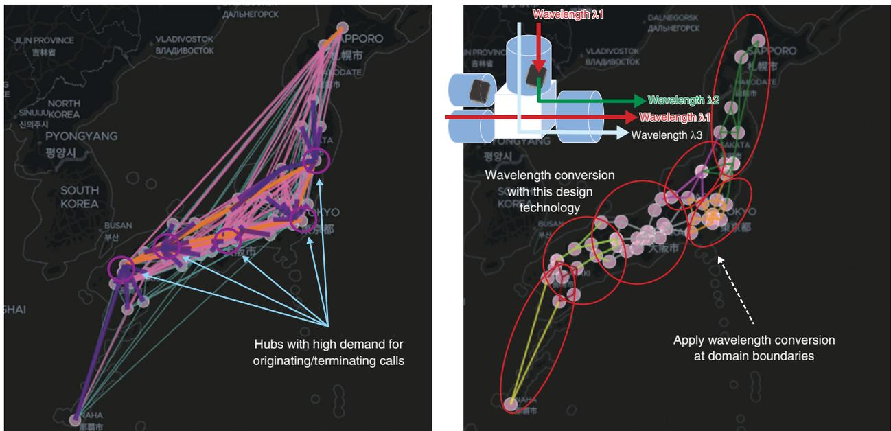
Domain configuration centered about hubs with high demand for originating/terminating calls
