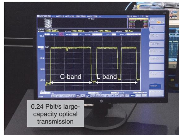
Fig. 2. Optical spectrum of large-capacity transmission system.
