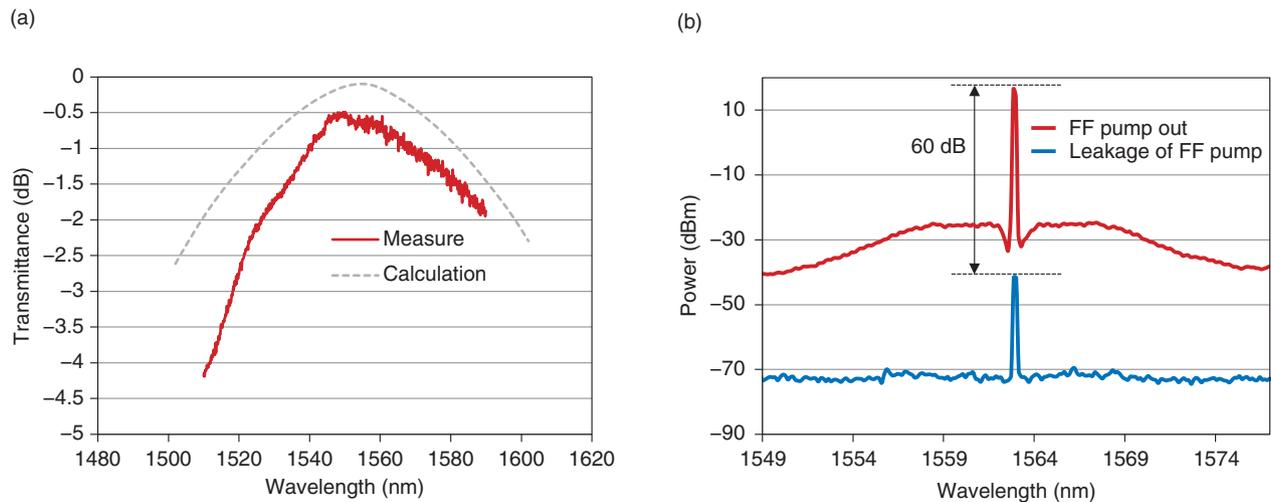
Fig. 2. (a) Transmittance of MMI for 1.56  $\mu\text{m}$  and (b) FF-pump isolation of WDM.
