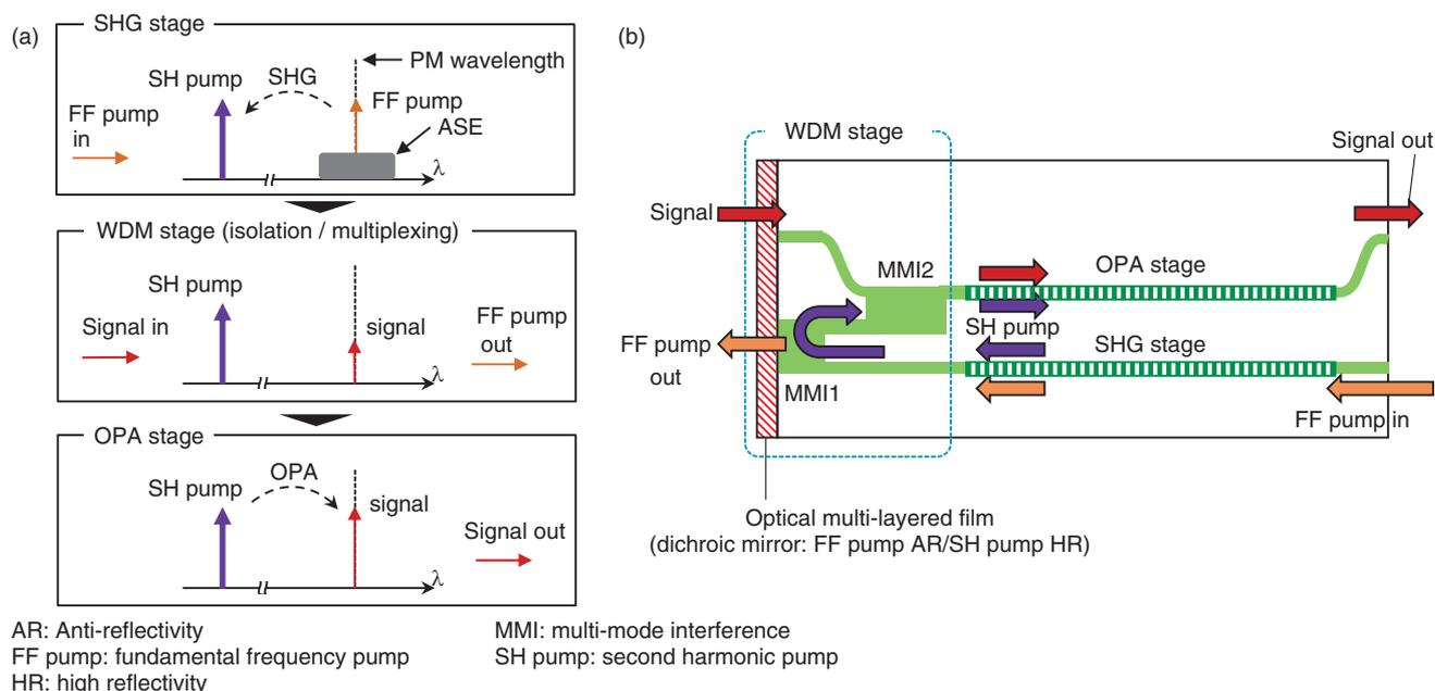
Fig. 1. (a) Operation flow of PPLN-based OPA and (b) schematic of integrated device.
