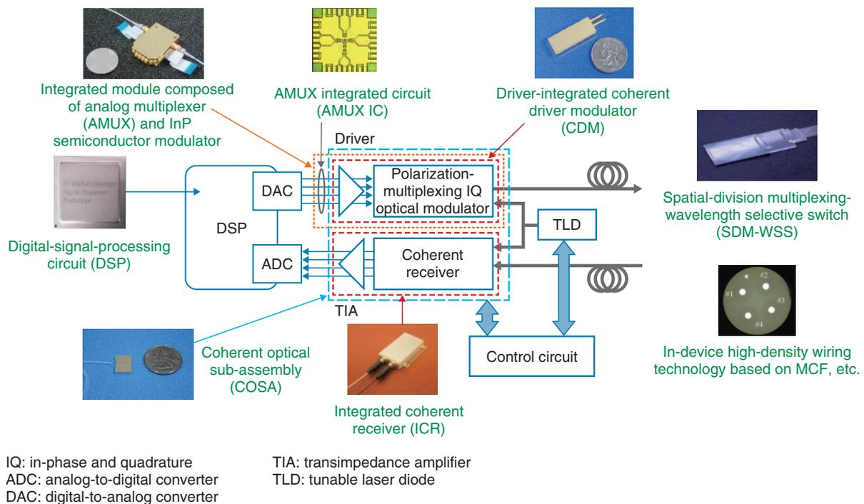
Fig. 3. Fundamental technologies for enabling 1-Tbit-class high-speed transmission.
