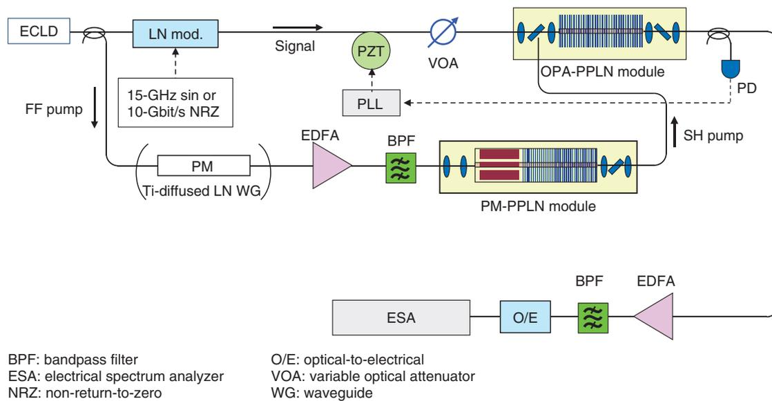
Fig. 7. Experimental setup for PSA using PM-PPLN module.
