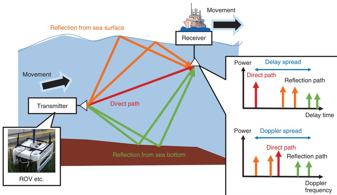
Fig. 2. Acoustic propagation through underwater channels.
