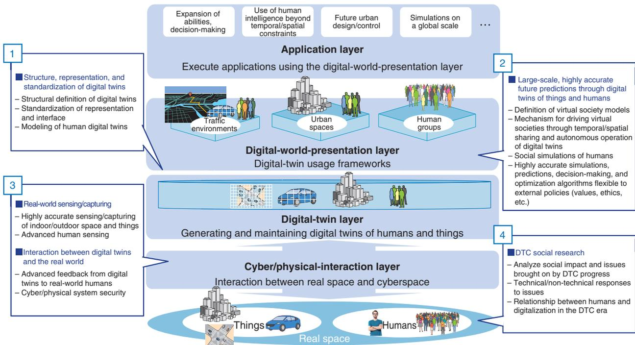
Fig. 3. DTC architecture and main issues surrounding implementation.
