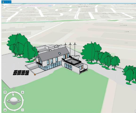
Building data of Autodesk Revit (a BIM tool) [1] (\*CC BY-NC-SA 3.0) are placed on the map by using Esri ArcGIS [2] (a GIS tool).
