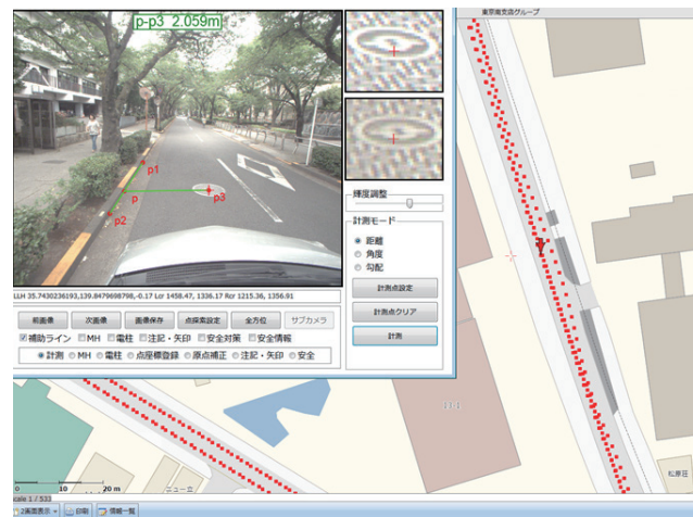
Fig. 1. 3D measurement from MMS images (vertical offset measurement from the pedestrian-road boundary to target facility).
