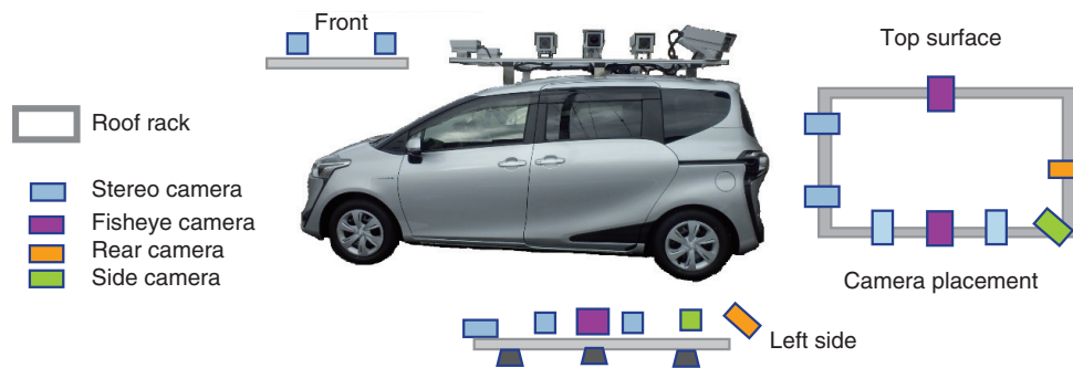
Fig. 2. Our MMS (camera placement).
