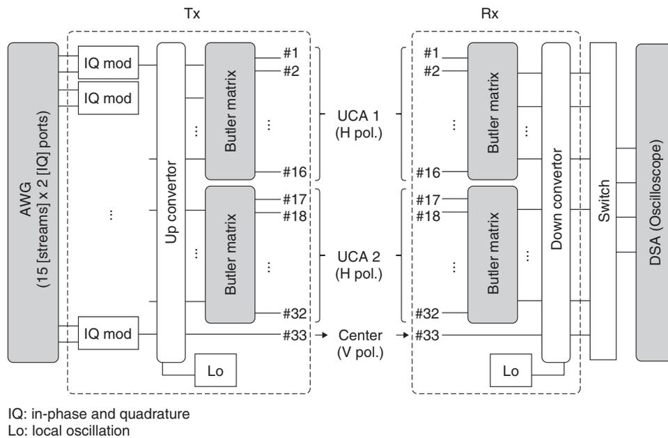
Fig. 6. Block diagram of our experiment.
