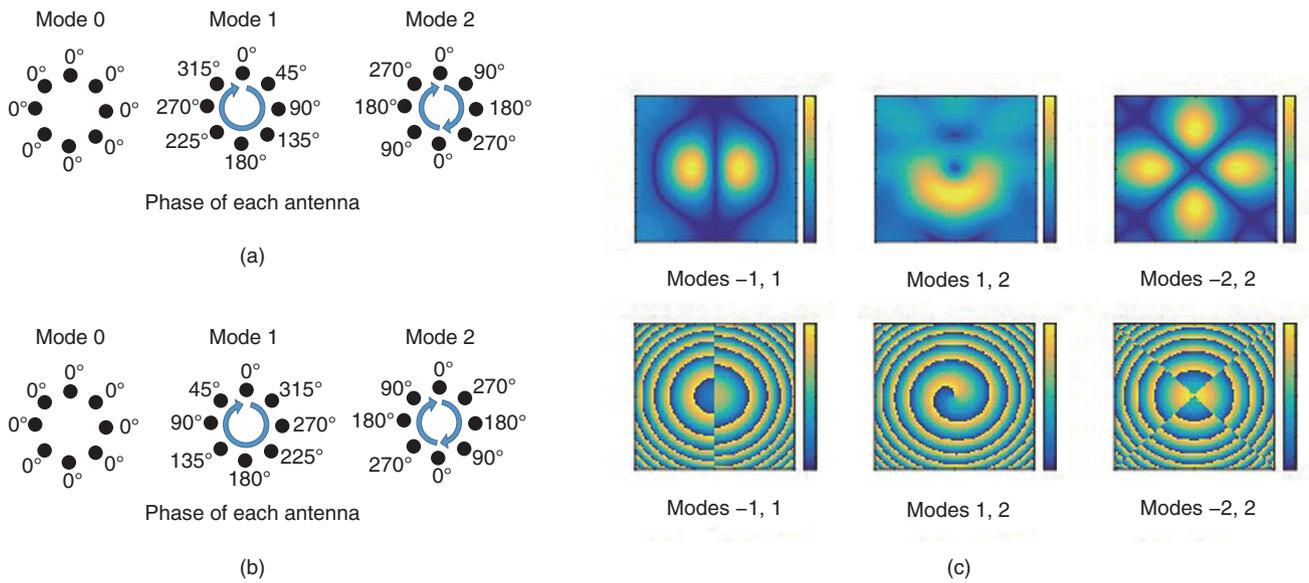
Fig. 3. (a) Generation of OAM modes with a UCA, (b) separation of OAM modes with a UCA, (c) intensity distribution (above) and phase distribution (below) of combined OAM modes ( $L$  is the number of OAM modes).
