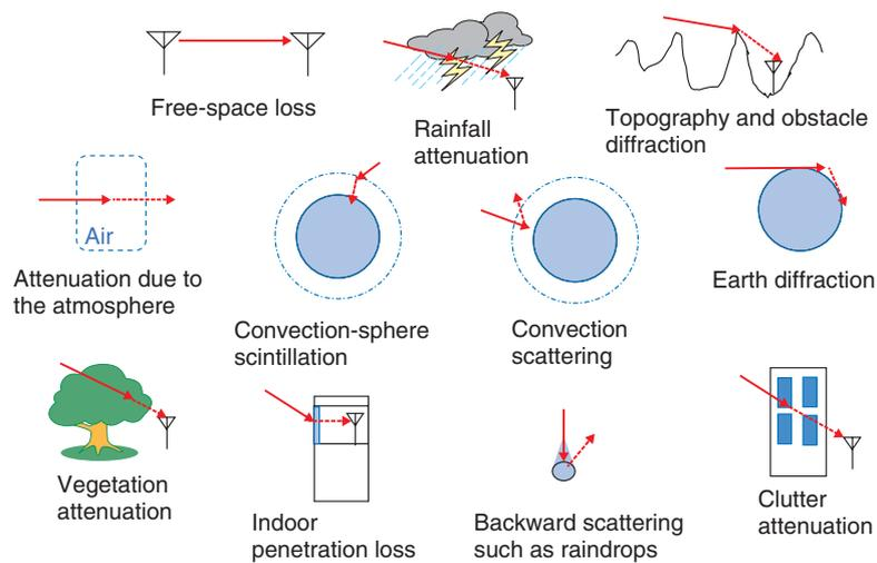
Fig. 2. Eleven propagation elements required for HIBS study.
