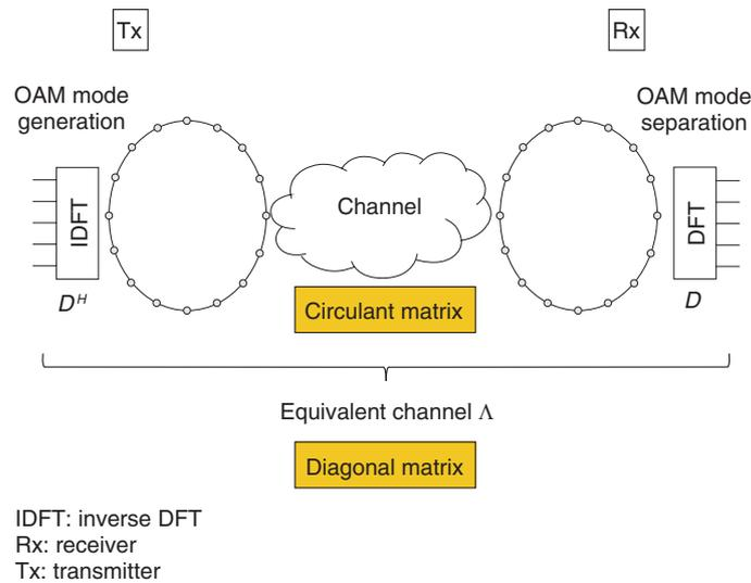
Fig. 4. Schematic of OAM multiplexing system.
