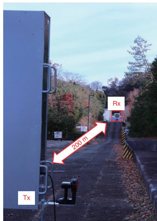
Fig. 8. Experimental environment for wireless OAM multiplexing transmission at a distance of 200 m in the field.
