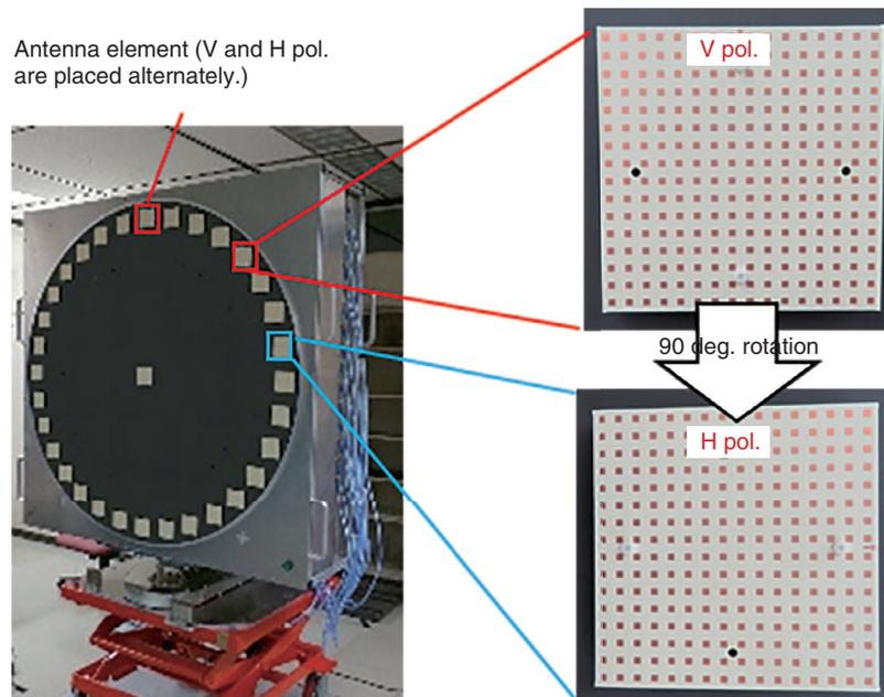
Fig. 5. Prototype of OAM transmission equipment.
