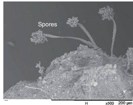
Fig. 4. Adhering substances on the walls. Top: optical-microscope image; bottom: SEM image.
