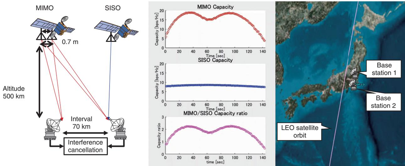
Fig. 4. Capacity enhancement using LEO-MIMO.
