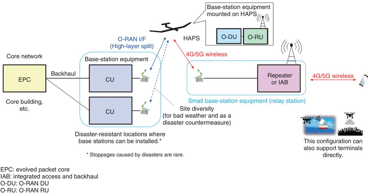
Fig. 2. Example of cooperative configuration when HAPS is used for backhaul.
