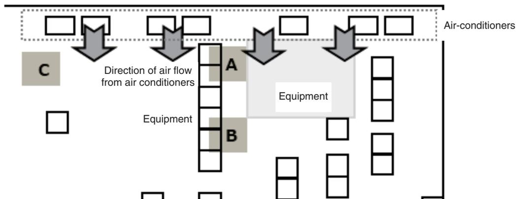
Fig. 5. Layout of equipment in machine room.
