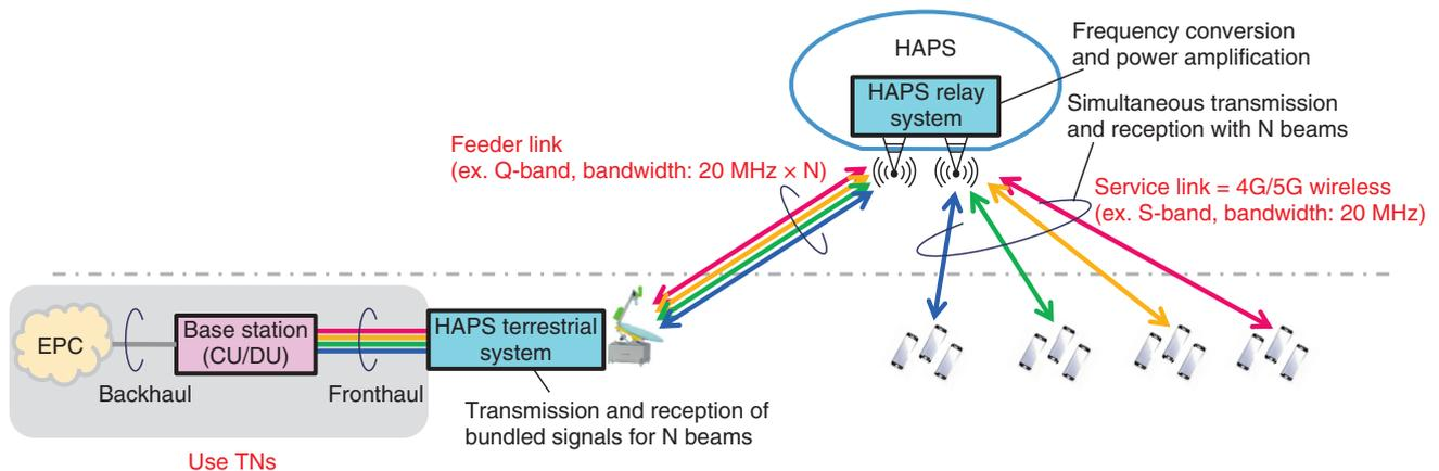
Fig. 3. Example of cooperative configuration when HAPS is used for direct access.
