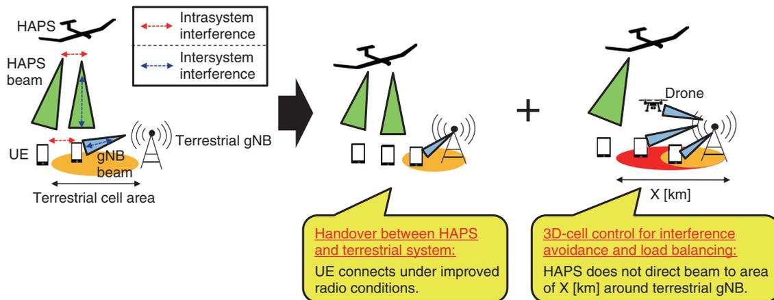
Fig. 4. Handover and 3D-cell control technology.
