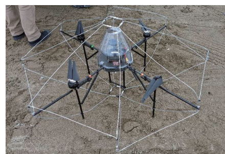
Fig. 2. Lightning-resistant drone under development.
