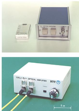
Fig. 1. World's first semiconductor-laser-pumped EDFA.
