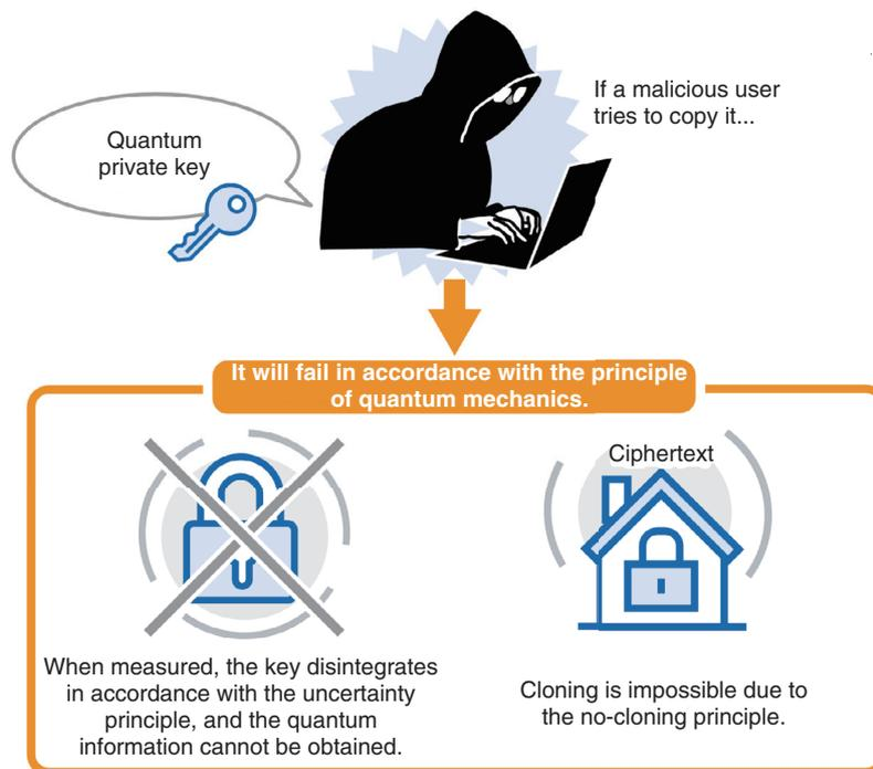
Fig. 4. Copy protection of a quantum private key.
