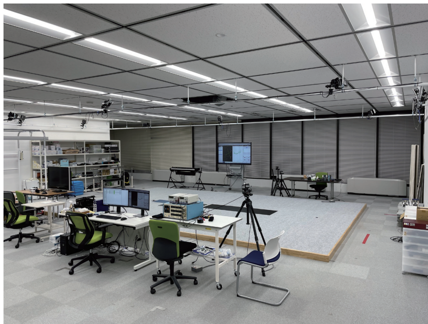
Fig. 2. Experimental facilities (measurement systems certified as medical equipment): VICON motion capture (11 cameras), DELSYS electromyography sensors, AMTI force plates, etc.
